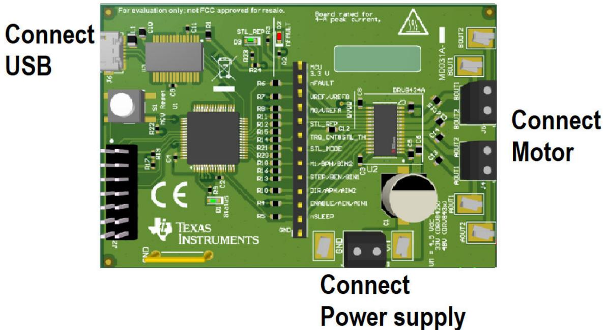
Figure 2-1. Board Connections
