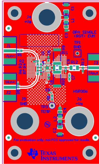
Figure 4. Top Components and Silk Screen Layer
