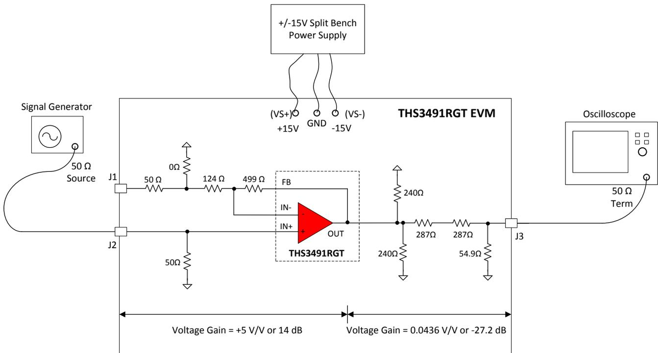
Figure 1. THS3491RGT EVM Default Configuration Setup Block Diagram
