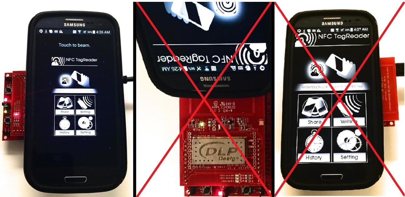
**Correct** - Phone NFC antenna presented over BoosterPack NFC antenna.
