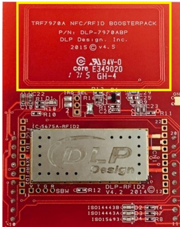
Figure 11. Antenna Location on DLP-7970ABP
