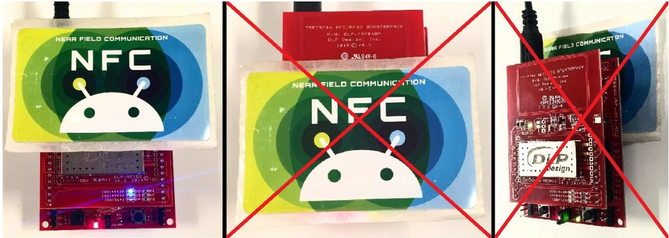
**Correct** - Tag presented on top of BoosterPack antenna.
