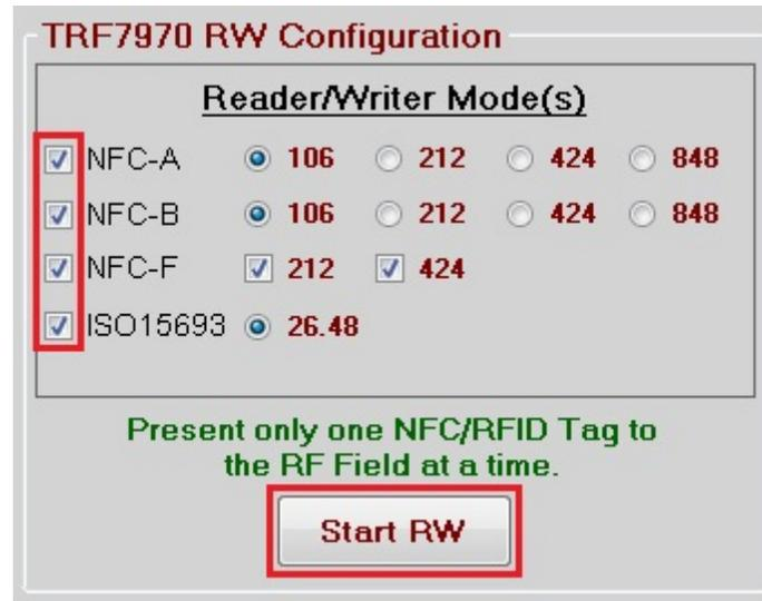
Figure 17. NFC Configuration Tab – RW Configuration
