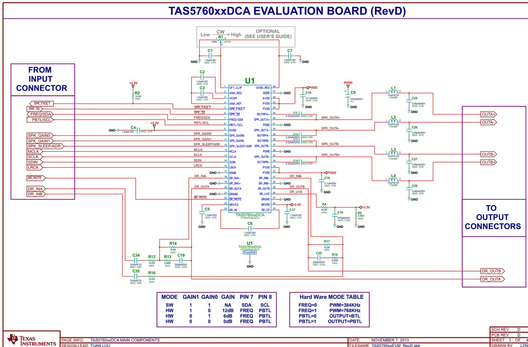
Figure 14. TAS5760xxEVM Rev D Schematic (Page 1 of 2)
