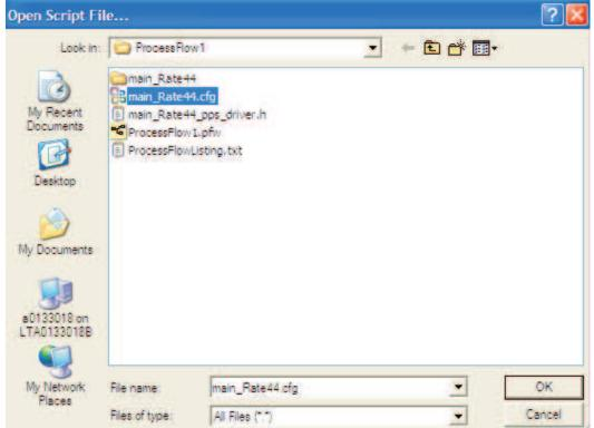
(e) Select the .cfg file in the Purepath™ Studio PS from /MiniDSPcode/ProcessFlow1/ folder.
