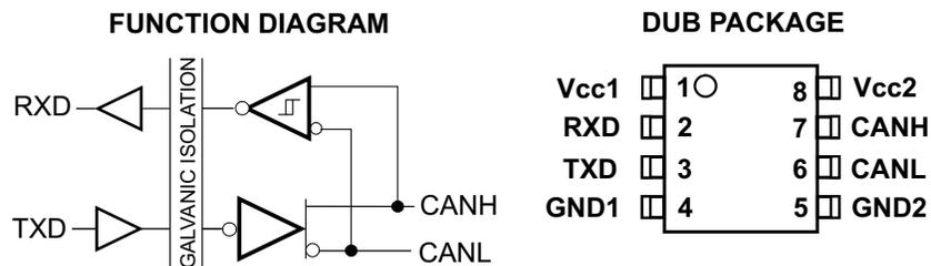
**Figure 1. The ISO1050 Function Diagram and Pinout**
