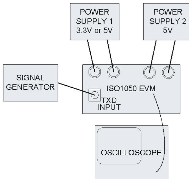
**Figure 4. Basic Isolated CAN Transceiver EVM Operation**
