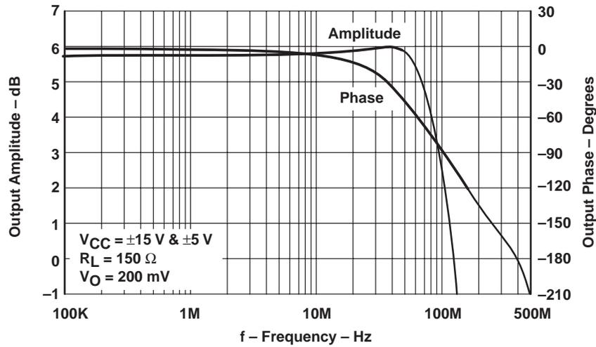
Figure 1–4 shows the typical frequency response of the THS4011 EVM using the inverting input ( $G = -1$ ). Typical  $-0.1$  dB bandwidths are 30 MHz and a  $-3$ -dB bandwidth of 83 MHz with a  $\pm 15$  V power supply. These bandwidths remain consistent when the power supply drops to  $\pm 5$  V.
