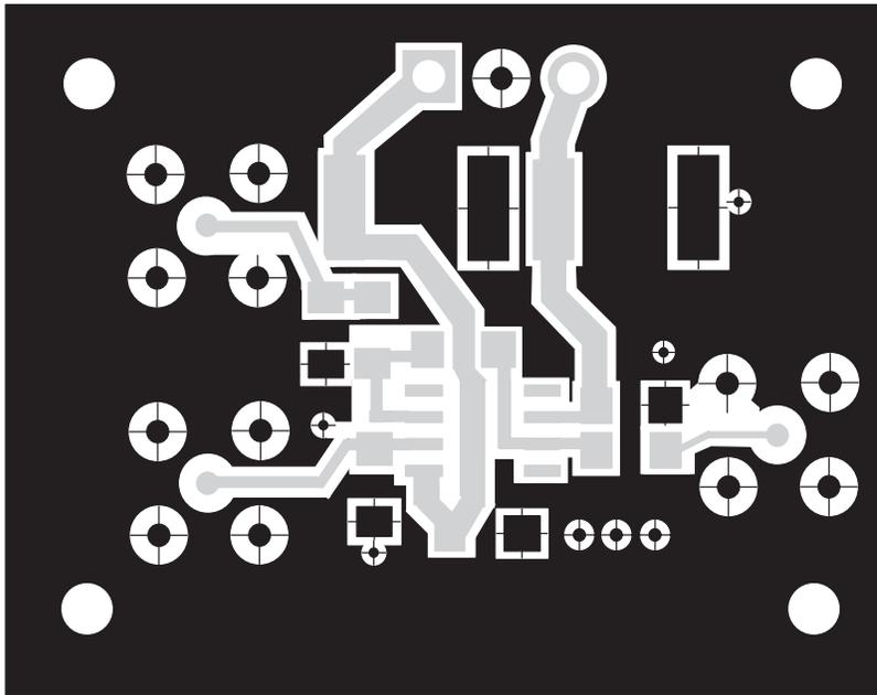
Figure 2–3. THS4011 EVM PC Board Layout – Back Side
