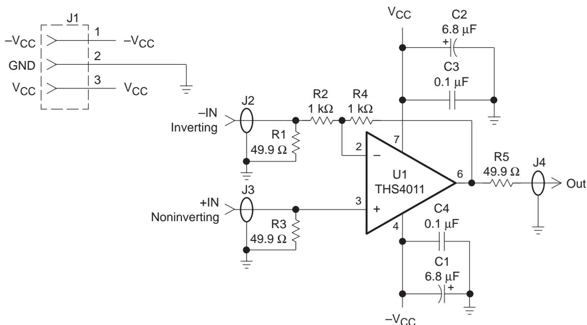
The gain of the EVM inputs can easily be changed to support a particular application by simply changing the ratio of resistors R1, R4, and R5 as described in the following equations:
