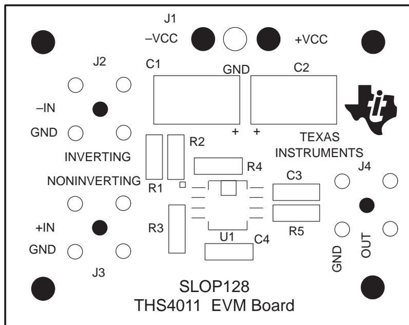
Figure 2–2. THS4011 EVM PC Board Layout – Component Side
