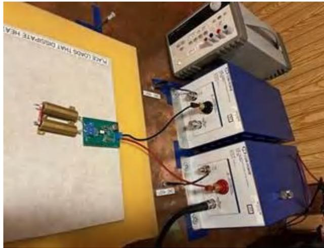
Figure 5-4. Conducted Emissions Test Setup
