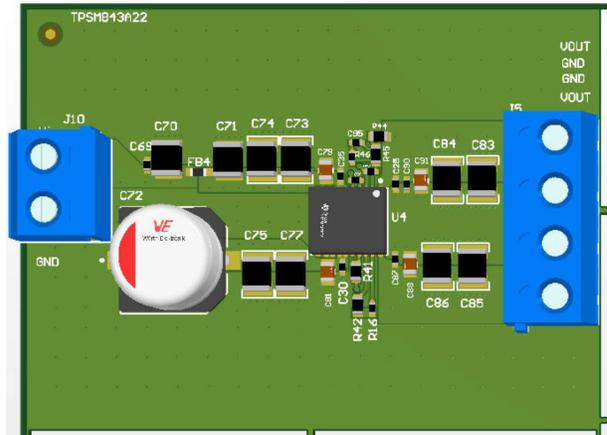
Figure 3-8. TPSM843A22 EMI-Optimized Layout
