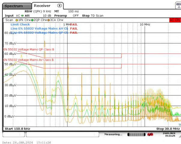
Figure 5-7. TPSM843620 Conducted EMI Results With Ferrite Bead Filter
