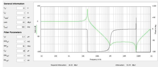
**Figure 5-3. Bode Plot for Inductor pi Filter**
