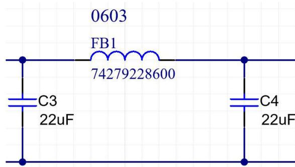
**Figure 5-1. Example pi Filter With Ferrite Bead**
