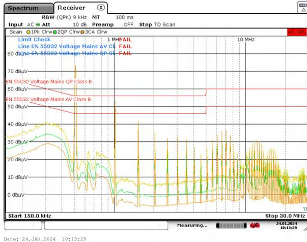
**Figure 5-11. TPSM843A22 Conducted EMI Results With Ferrite Bead Filter**
