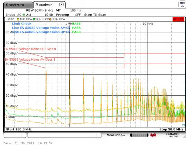
**Figure 5-12. TPSM843A22 Conducted EMI Results With Inductor Filter**
