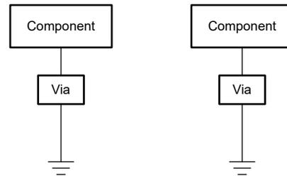
Figure 2-2. Avoided Ground Loop Connection With Vias
