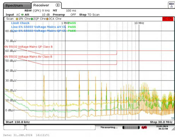
Figure 5-6. TPS543820 Conducted EMI Results With Inductor Filter
