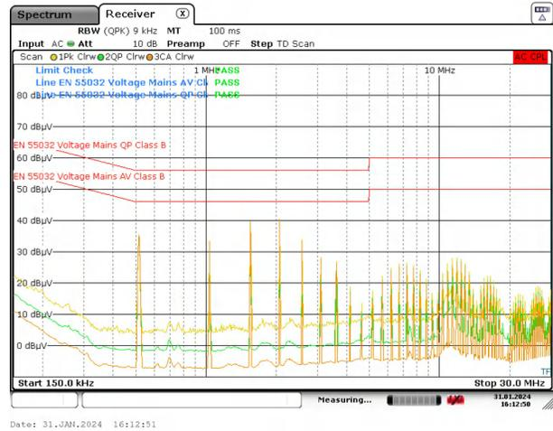
**Figure 5-10. TPS543A22 Conducted EMI Results With Inductor Filter**
