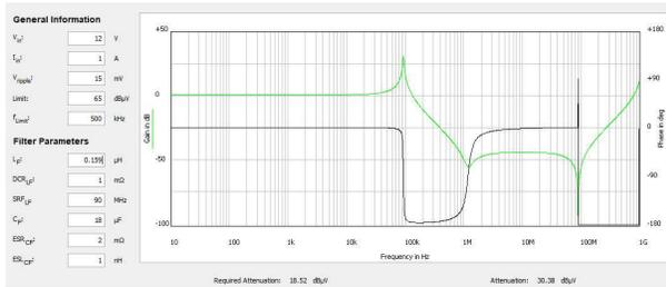
**Figure 5-2. Bode Plot for Ferrite Bead pi Filter**
