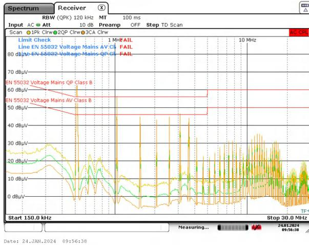
**Figure 5-9. TPS543A22 Conducted EMI Results With Ferrite Bead Filter**
