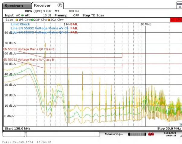
Figure 5-5. TPS543820 Conducted EMI Results With Ferrite Bead Filter
