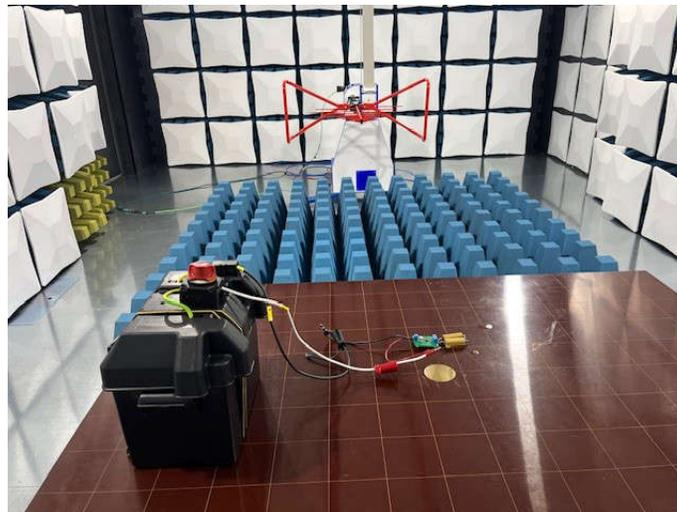
Figure 4-1. Radiated Emissions Testing Setup
