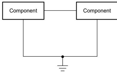
Figure 2-1. Ground Loop Connection
