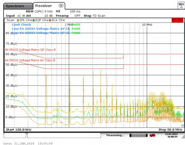
Figure 5-8. TPSM843620 Conducted EMI Results With Inductor Filter
