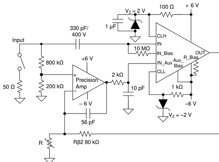
Figure 1. Example BUF802 Composite Loop Configuration
