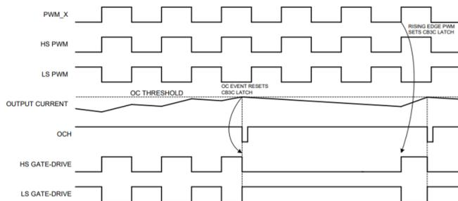
Figure 1. CBC Timing Diagram for Automotive Class-D Audio Amps
