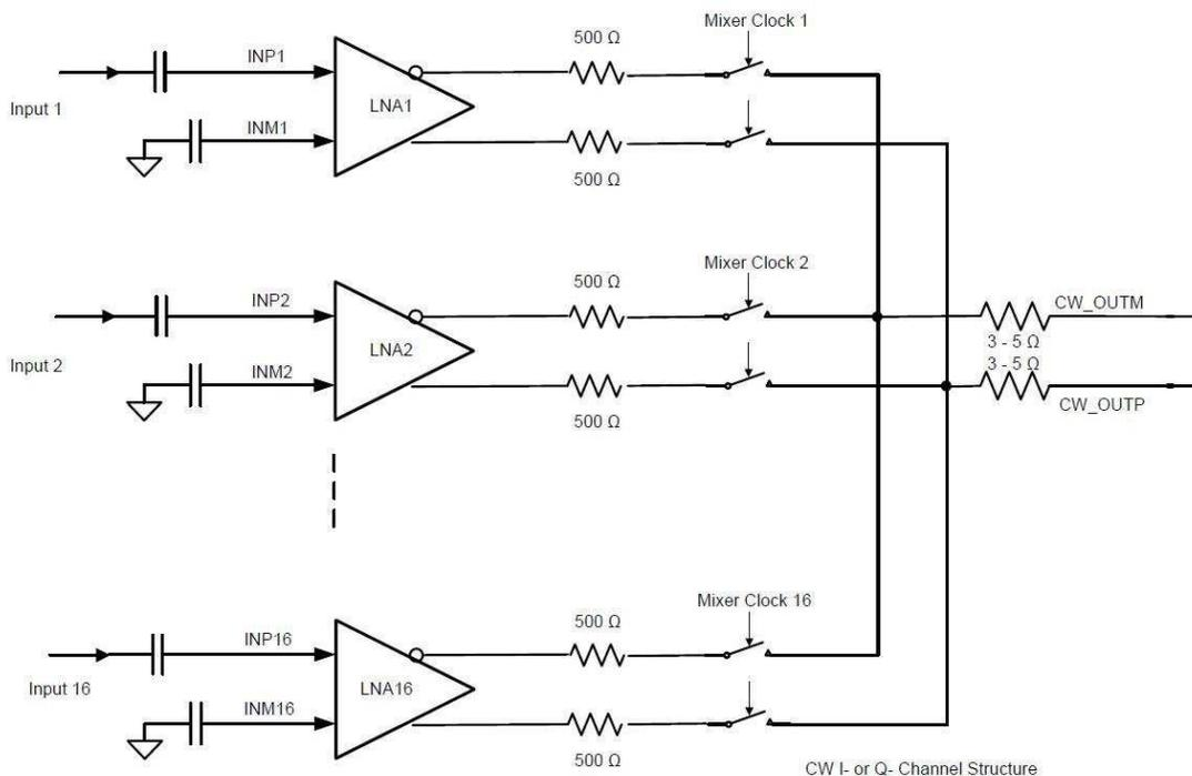
NOTE: The 3-Ω to 6-Ω resistors at CW\_OUTP and CW\_OUTM result from the internal device routing and can create a slight attenuation in the signal.
