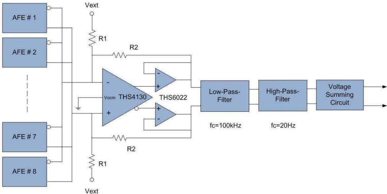
**Figure 3. Using Buffer to Improve the Output Current Sink/Source Capability of THS4130**
