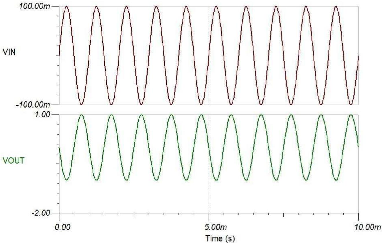
Figure 5. Output Waveform for Circuit Using Buffer
