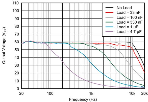
Figure 2. Amp Gain Bandwidth VBST 30 V
