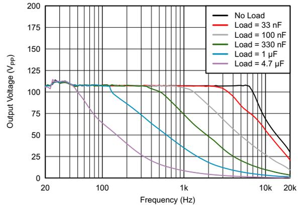
Figure 3. Am Gain Bandwidth VBST 55 V
