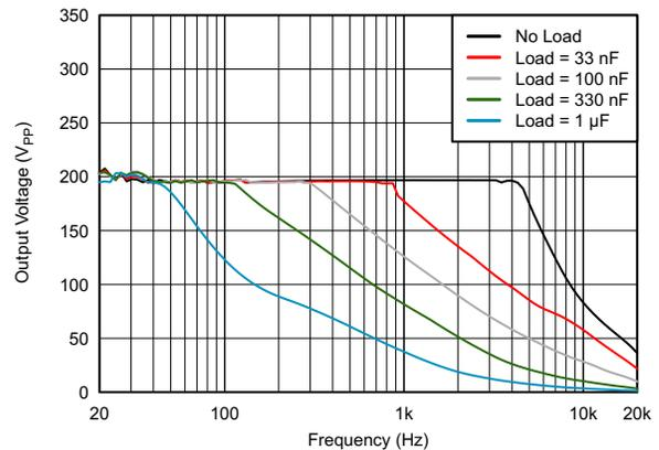
Figure 5. Amp Gain Bandwidth VBST 105 V
