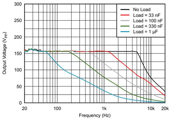
Figure 4. Amp Gain Bandwidth VBST 80 V
