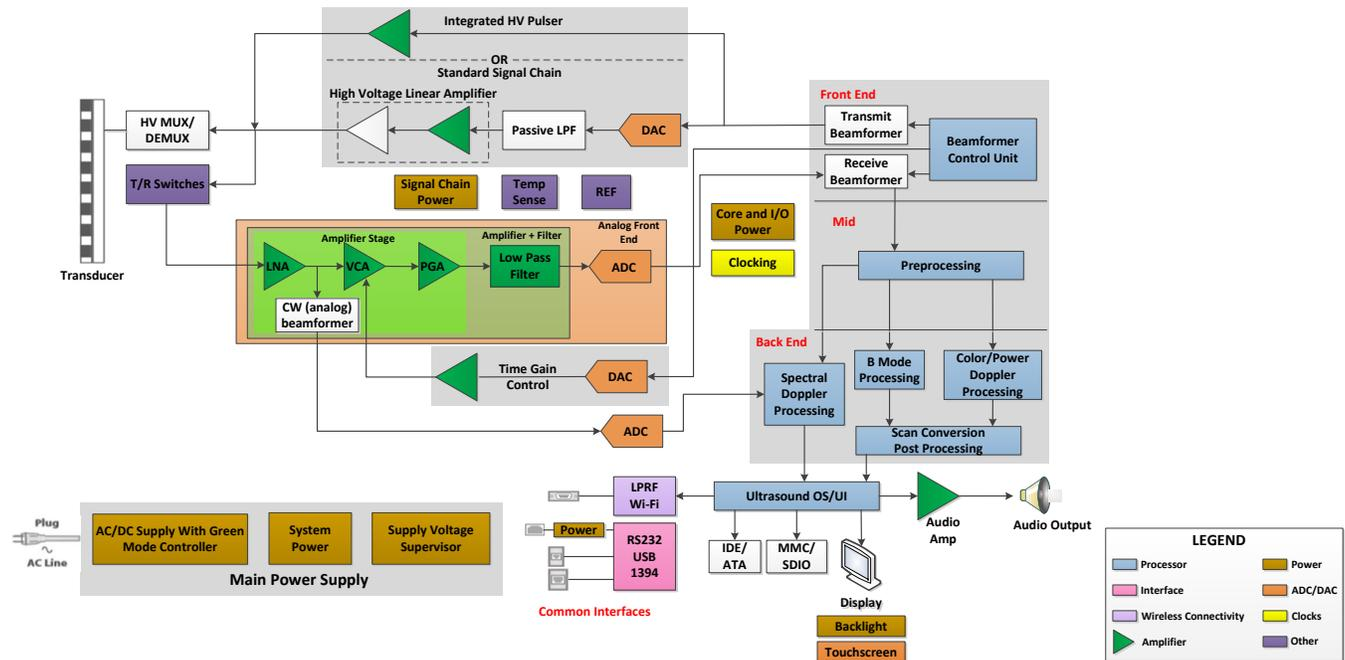
The following image shows TI's AFE5818 signal chain and how it connects to the rest of the ultrasound topology (denoted by the red arrows).
