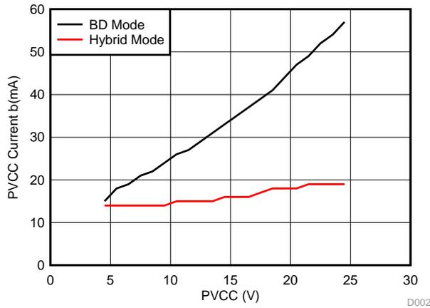
Figure 2. PVCC Idle Current vs. Voltage Without Snubber
