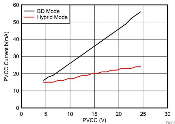
**Figure 1. PVCC Idle Current vs. Voltage With Snubber**
