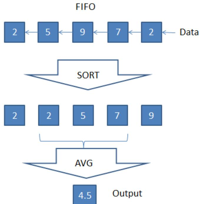
**Figure 3. Median Average Filter Operation**
