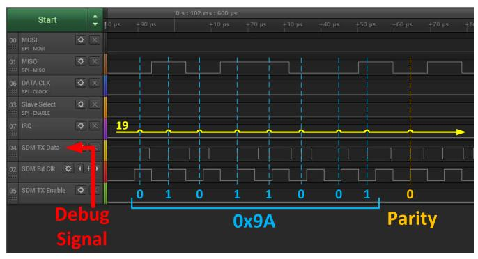
Figure 11. Receiving in Direct Mode 1
