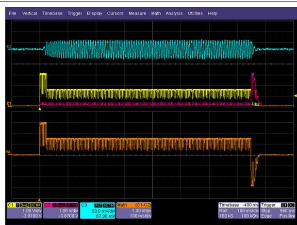
Figure 3-3. Typical ERM Alert Effect With TI's Closed-Loop Driver
