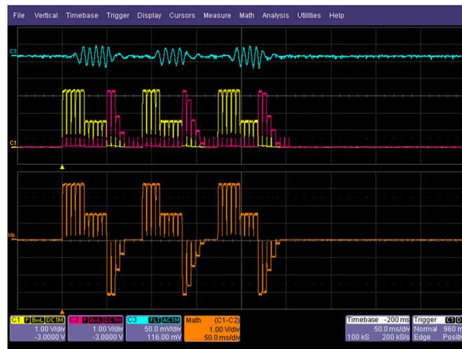
Figure 4-8. ERM Triple Click Waveform - NRS2574i
