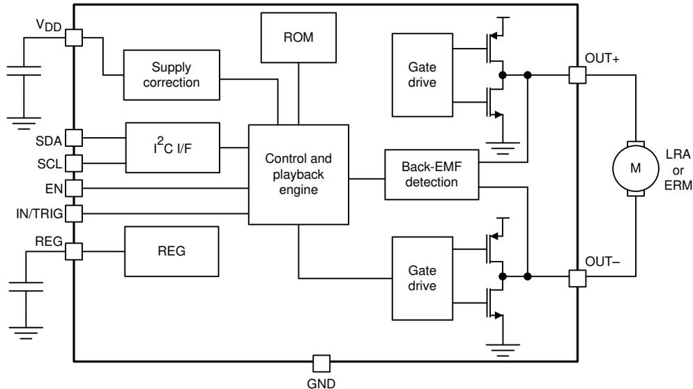
Figure 2-1. DRV2605 Block Diagram
