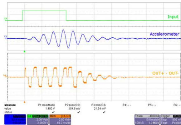
Figure 5-3. Click with Braking
