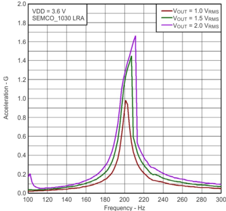
**Figure 3-1. Resonant Frequency of Linear Resonant Actuators**
