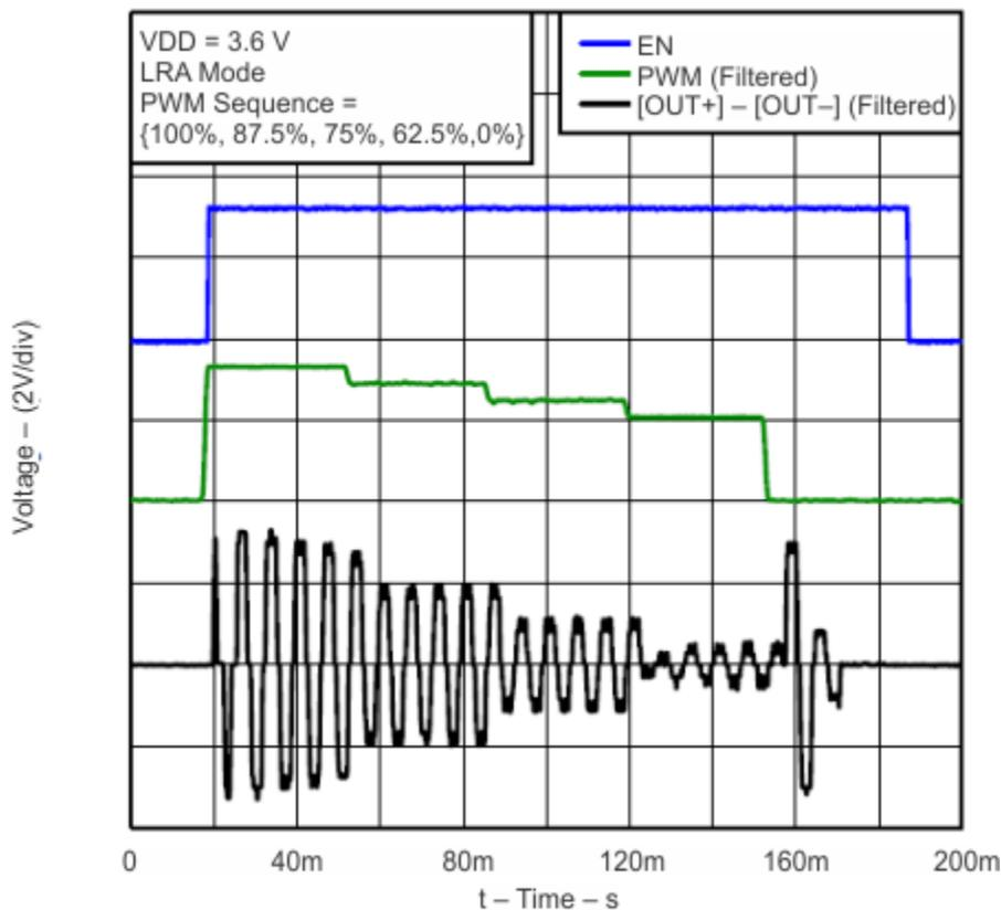
**Figure 1-1. LRA Auto-Resonance Detection**
