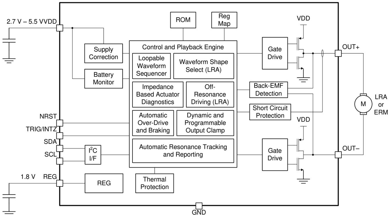
Figure 2-2. DRV2625 Block Diagram
