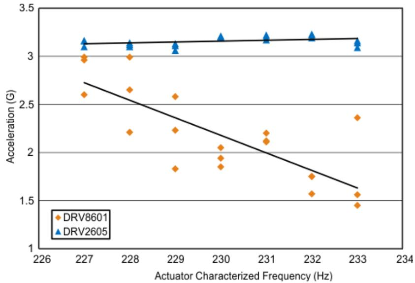
**Figure 3-2. Acceleration Performance of the DRV2605 versus DRV8601**
