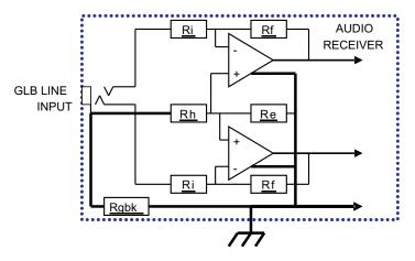
Again, a GLB input may be implemented with an audio subsystem, codec or other device with an available mono input that can be summed to its outputs. It is simply necessary to connect this input to the junction of Rgbk and the input jack sleeve and set its gain to the outputs to -1 times channel gain.
