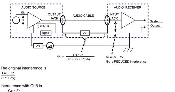
So the modified circuit reduces interference by the following ratio.
