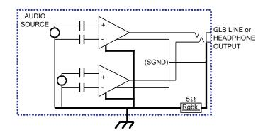
This circuit may be implemented very easily with Texas Instruments' TPA6132A2 or several other devices in the TPA613x family. An implementation with TPA6132A2 is shown in Appendix A. These devices are good choices for GLB circuits because they provide compact, integrated solutions with high CMRR. Members of the DRV60x family and TPA4411 are also good candidates for use in GLB output circuits. (For additional implementations of GLB circuits, see Appendix B.)
