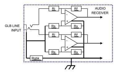
As before, in many cases it is not necessary or possible to use separate resistor chains at the non-inverting inputs of the opamps, and they are combined into one chain. In this case the circuit must invert the input signal, because the opamp feedback chains must be distinct. Circuit gain is (Rf/Ri). Again, the resistors in the combined chain, Rh and Re, must have the same ratio as Ri and Rf, but their values do not have to be the same.
