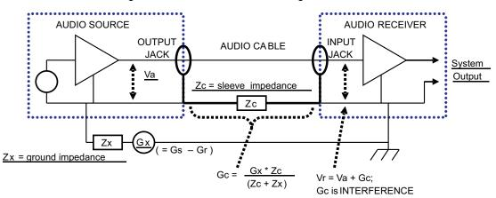
Gc, part of the ground potential Gx, appears across the audio jack sleeve contacts and the audio cable shield, adding interference to the input to the receiver. Reducing this requires 2 steps.
