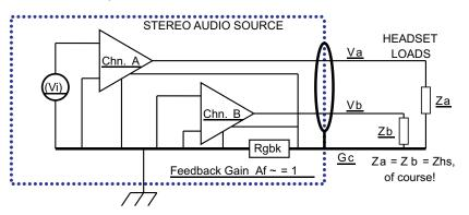
Feedback gain Af from Rgbk back through the amplifiers to their outputs is intended to be exactly 1, to offset voltage across Rgbk. But Af has some error. If this error is small, there will be no problem, but if it is large, Rgbk will create crosstalk.
