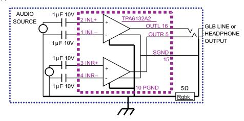
TPA6132A2 and other devices with SGND in the TPA613x family are well suited for this application because they provide a small, highly integrated solution with high-CMRR differential amplifiers. Since the differential amplifiers are completely integrated into the device, there are no resistors except Rgbk to add to TPA6132A2 to complete a GLB output, and the inherent high CMRR of the differential amplifiers prevents crosstalk problems.
