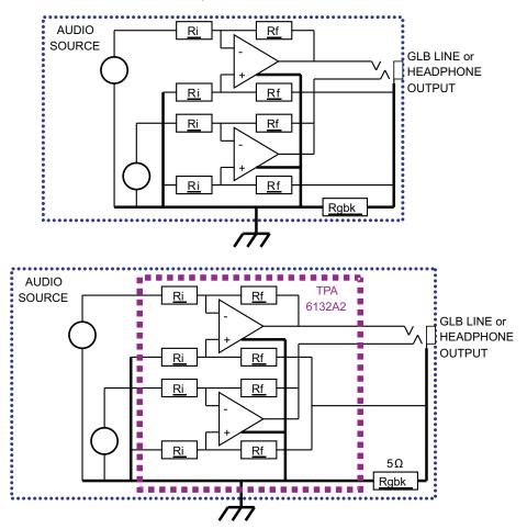
TI devices like TPA6132A2, DRV602, DRV603, DRV604 make good candidates for use in GLB output circuits.
