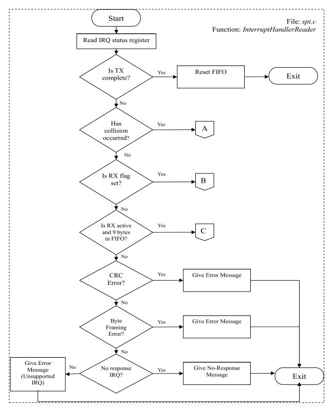
Figure 2. Inerrupt Handler Routine (1)
