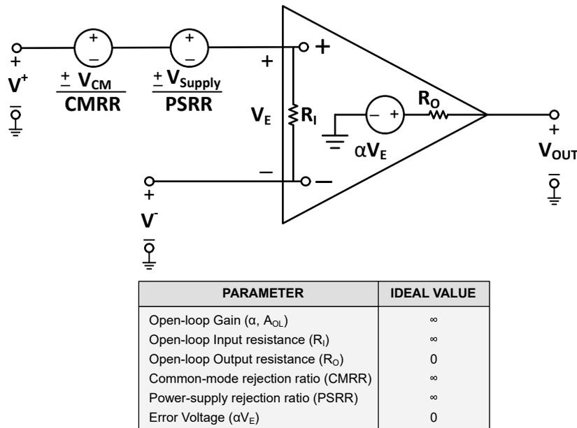
**Figure 1-1. Ideal Op Amp Model and Model Parameters**
