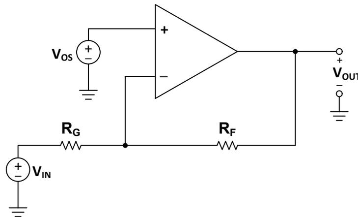
**Figure 6-1. Inverting Op Amp Circuit With  $V_{OS}$  Included**
