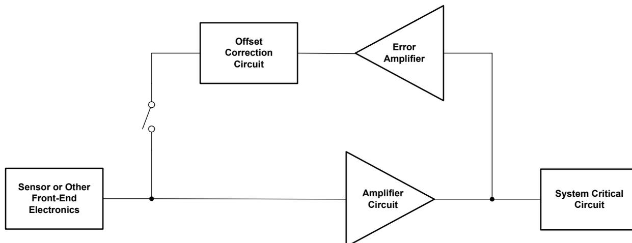
**Figure 6-3. General Form of DC Feedback Loop**
