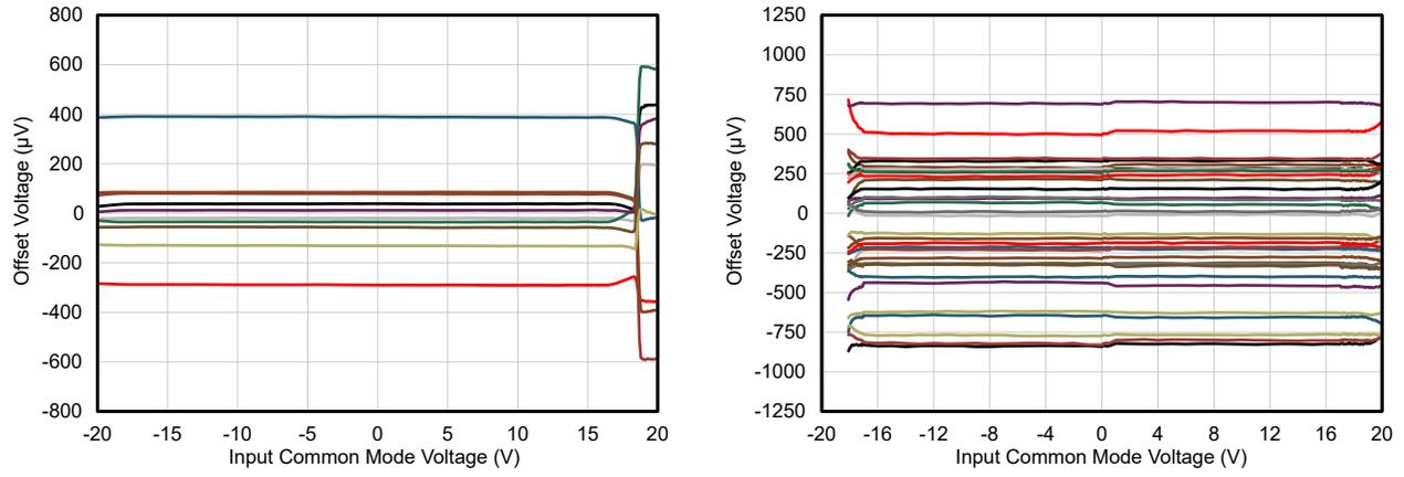
**Figure 5-4.  $V_{OS}$  vs.  $V_{CM}$  for the OPAx991 (Left) and the TL07xH (Right)**
