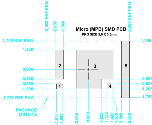
Figure 2. Micro (MPB) - Solder Mask Defined PCB Recommended Layout
