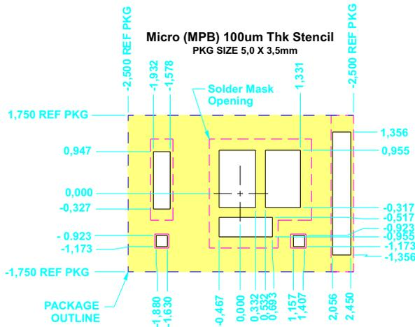
**Figure 5. Micro (MPB) – 100µm Stencil Thickness Recommended Layout**
