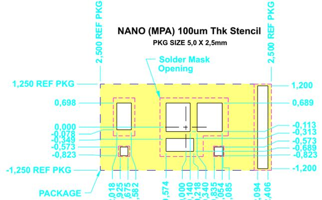
**Figure 8. Nano (MPA) – 80µm Stencil Thickness Recommended Layout**
