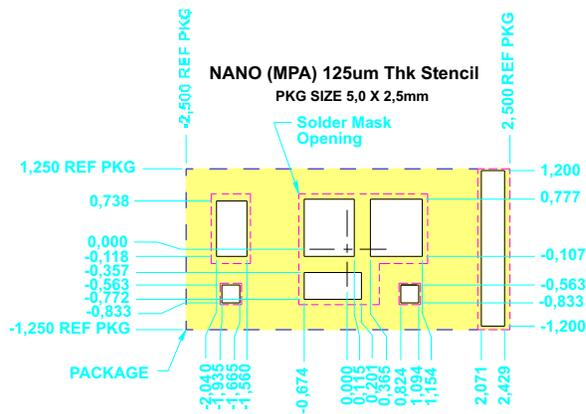
**Figure 9. Nano (MPA) – 125µm Stencil Thickness Recommended Layout**
