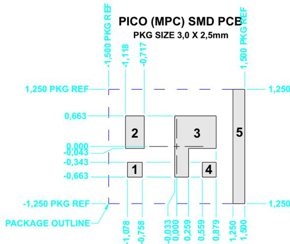
Figure 4. Pico (MPC) - Solder Mask Defined PCB Recommended Layout
