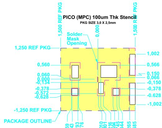
**Figure 10. Pico (MPC) – 100µm Stencil Thickness Recommended Layout**
