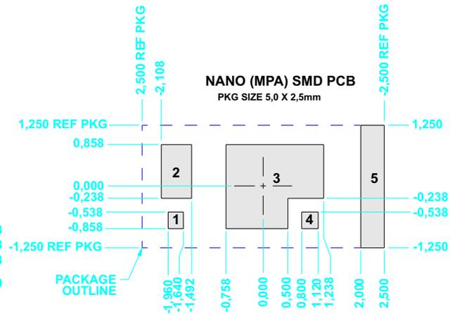
Figure 3. Nano (MPA) - Solder Mask Defined PCB Recommended Layout
