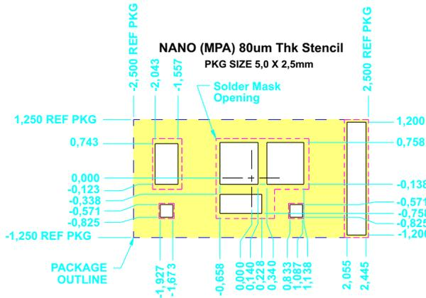
**Figure 7. Nano (MPA) – 80µm Stencil Thickness Recommended Layout**
