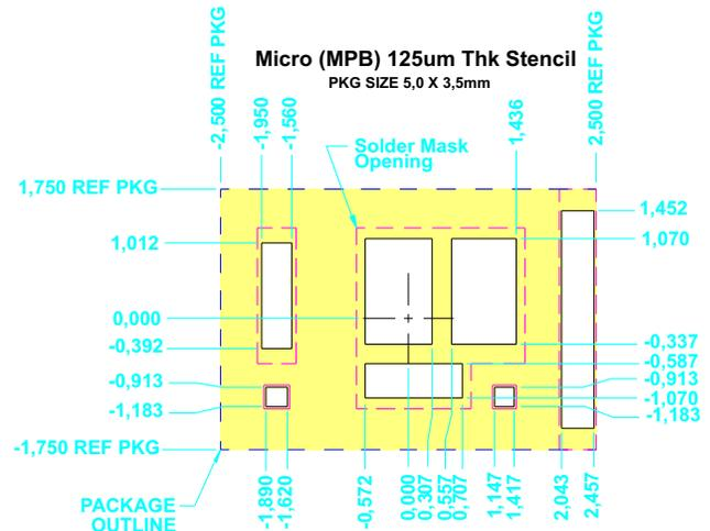
**Figure 6. Micro (MPB) – 125µm Stencil Thickness Recommended Layout**
