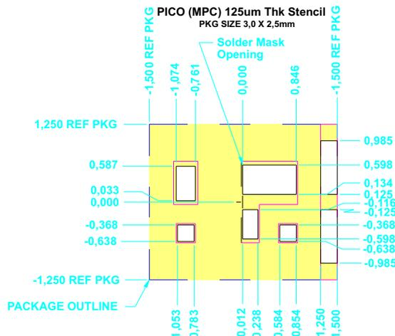
**Figure 11. Pico (MPC) – 125µm Stencil Thickness Recommended Layout**
