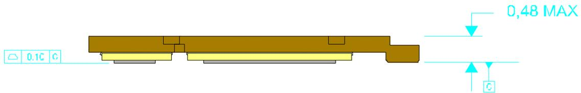
**Figure 1. Power Block II Package Illustrated Cross-Section**
