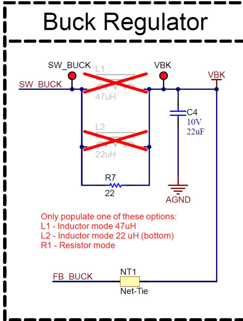
Figure 4-7. Buck Regulator Schematic
