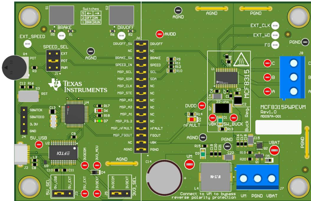
MCF8315PWPEVM Printed Circuit Board (PCB - Top View)
