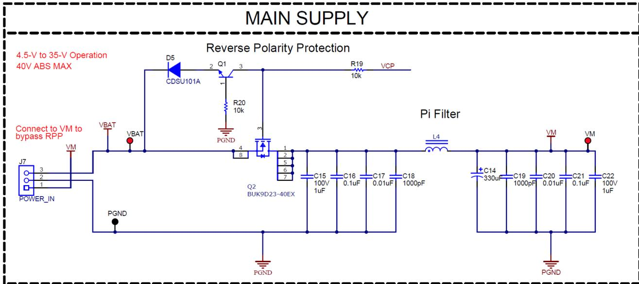
Figure 4-1. Main Supply and Pi Filter Schematic
