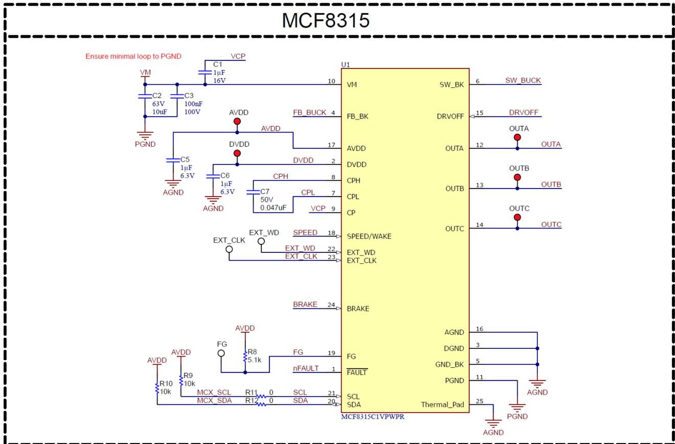
Figure 4-6. MCF8315 3-Phase Sensorless FOC Integrated Driver Schematic
