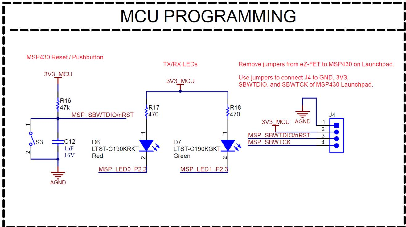
Figure 4-4. MCU Programming and Debug Schematic
