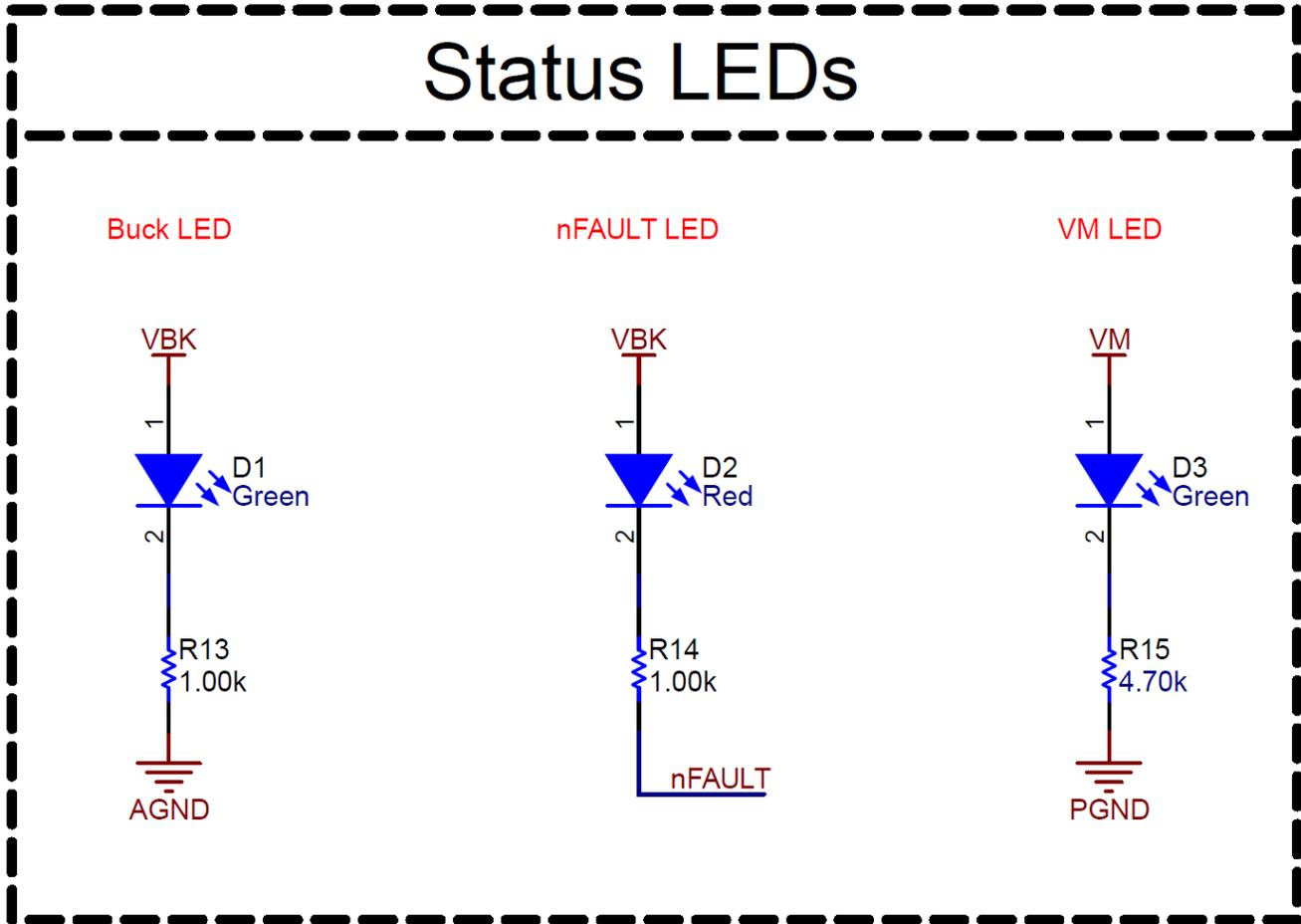
Figure 4-8. Status LEDs Schematic
