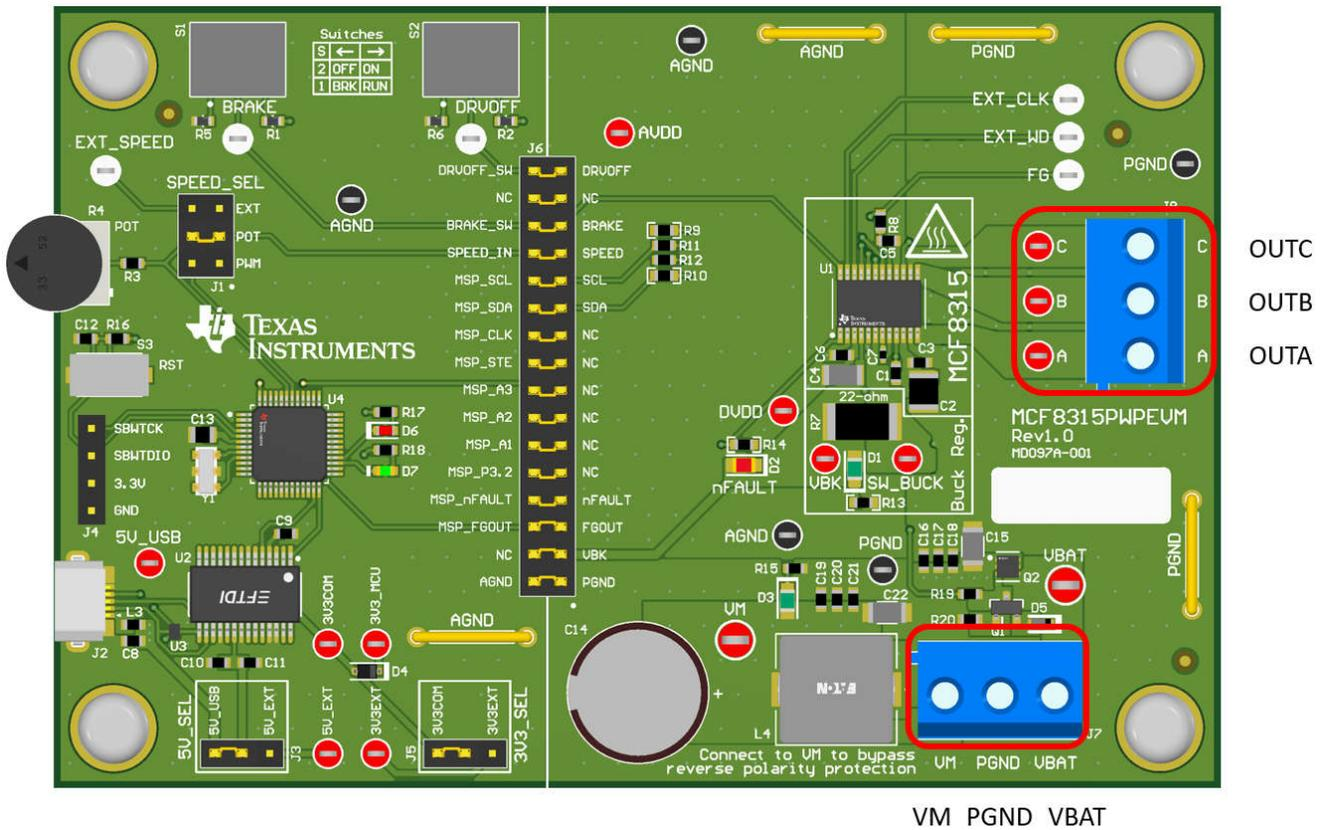
Figure 2-3. Connections from Motor to MCF8315PWPEVM
