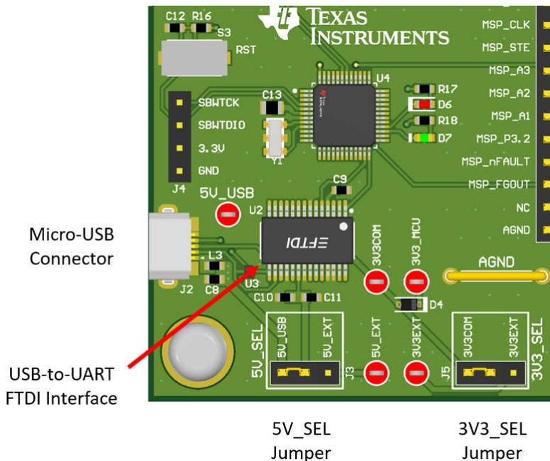
Figure 2-4. Micro-USB Connector and UART for MCF8315PWPEVM
