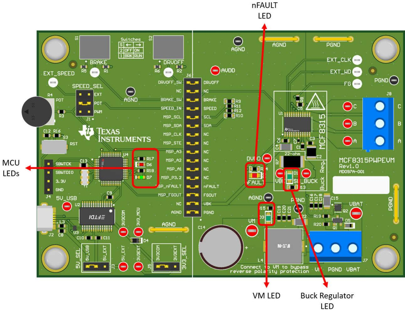
**Figure 2-6. MCF8315PWPEVM LEDs**
