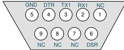
Figure 3-2. Female DB9 Connector Pinout
