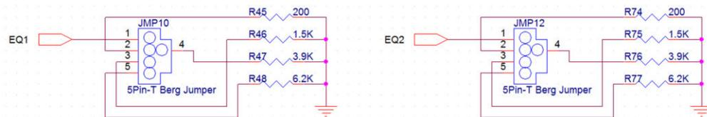
**Figure 2-3. Early Board JMP10 and JMP12 Schematic**
