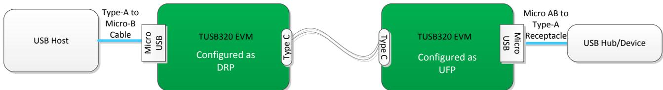
Figure 3. Example Configuration Using HD3SS2522 and TUSB320 EVMs
