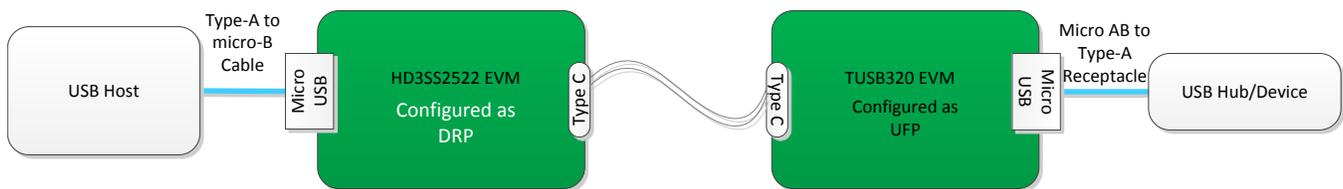
Figure 1. Example Configuration Using HD3SS2522 and TUSB320 EVMs
