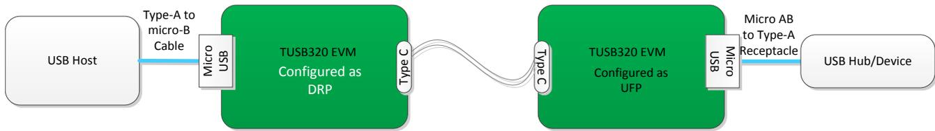
**Figure 4. Example Configuration Using Two TUSB320 EVMs**
