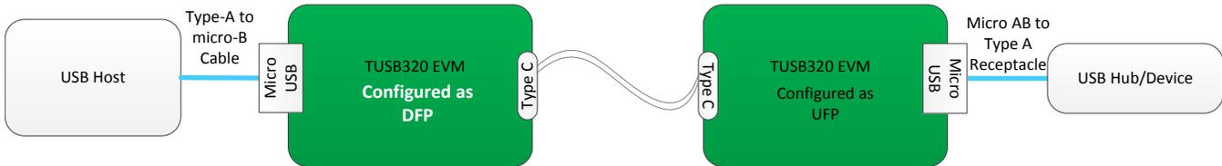
Figure 2. Example Configuration Using Two TUSB320 EVMs
