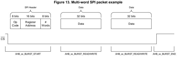
Figure 13 shows a 2 word SPI transfer example, and how the READ/WRITE function is called twice to do each individual word transfer. This is helpful for cutting down on the SPI overhead when transferring a CAN message to or from the TCAN4550-Q1, and minimize the maximum SPI frequency required.
