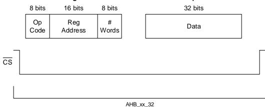
Figure 11. 32-bit SPI read or write example
