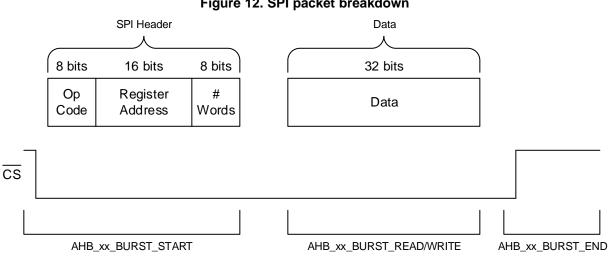
Figure 12. SPI packet breakdown
