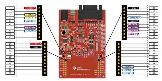
The BoosterPack kit adheres to the 40-pin LaunchPad and BoosterPack pinout standard. This standard was created to aid compatibility between LaunchPad development kit and BoosterPack module tools across the TI ecosystem.
