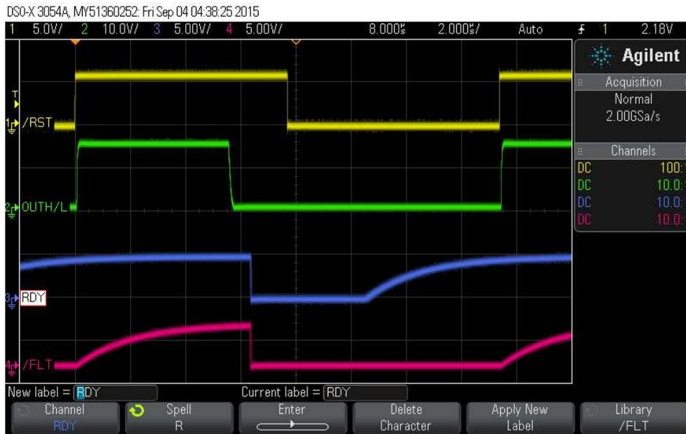
Figure 7. ISO5852S EVM OUTH/L, RDY, FLT, and RST With Unipolar Output Supply
