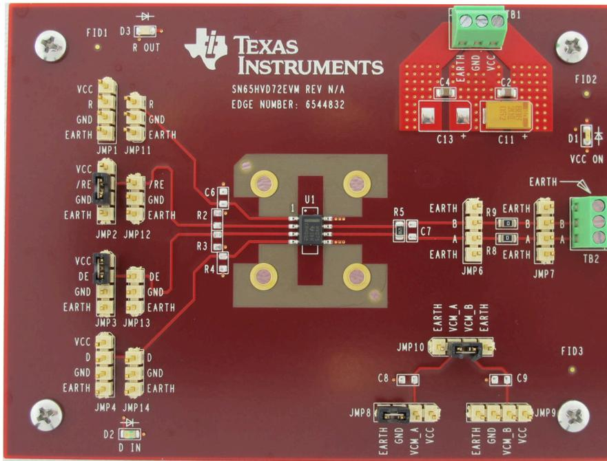
**Figure 4-6. Top View of RS-485 Half-Duplex EVM**
