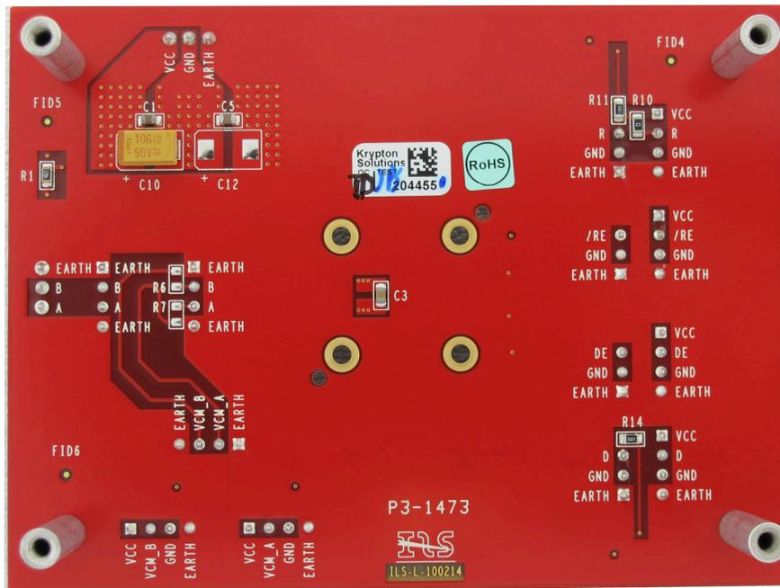
**Figure 4-7. Bottom View of RS-485 Half-Duplex EVM**
