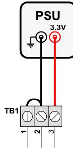
**Figure 3-2. Bridging DUT\_GND with EARTH\_GND**
