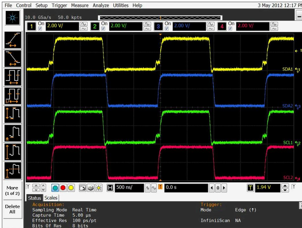
Note the  $t_{LOOP}$  effect on the rising edge of the input waveforms on SDA1 and SCL1.
