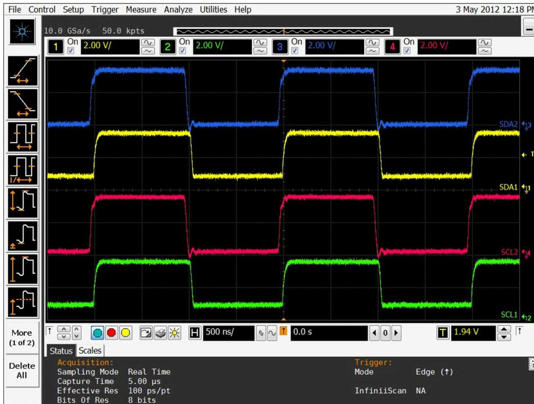
Note the offset of the output low level voltage from ground on SDA1 and SCL1.
