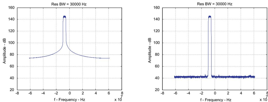
Figure 23. Comparison of Using the Exact Frequency (left) vs Rounded Frequency (right)
