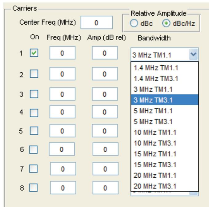
Figure 33. Specific LTE Bandwidths Available for Testing
