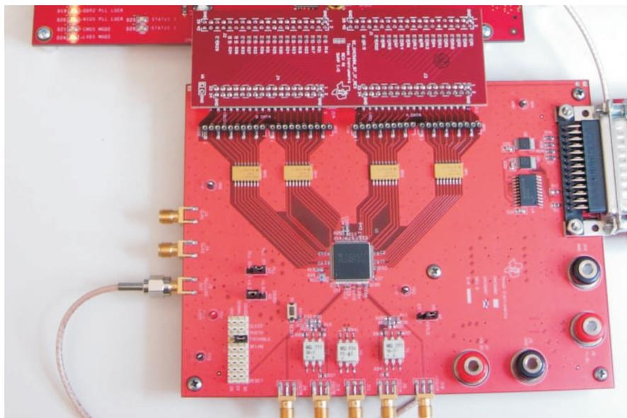
**Figure 14. CMOS HSDAC Connection to the TSW3100**
