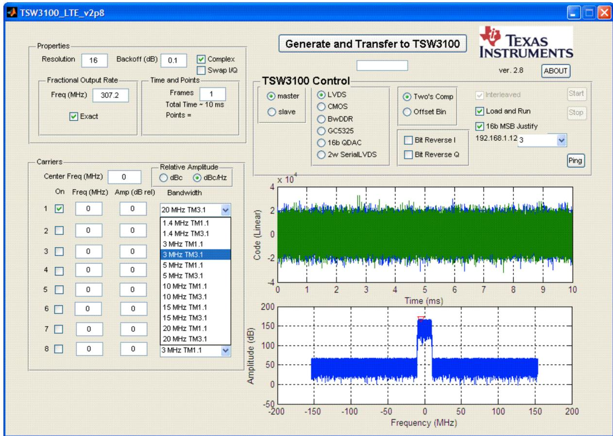
Figure 32. LTE Bandwidth Selection Within GUI
