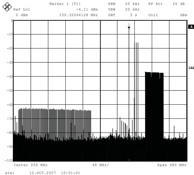
**Figure 19. DAC5682Z Output Spectrum for Four Tone Groups**
