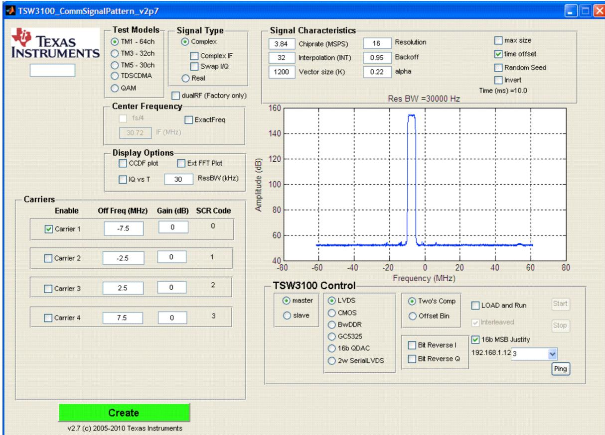
Figure 22. TSW3100\_CommSignalPattern Graphical User Interface
