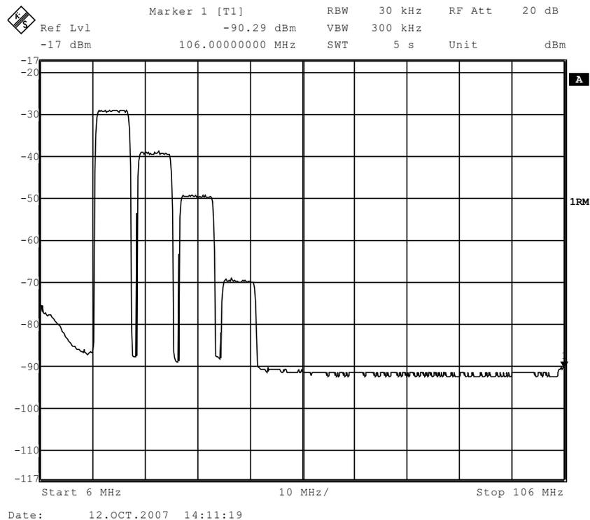
Figure 30. DAC5687 Output Spectrum for Four-Carrier QAM256 Pattern
