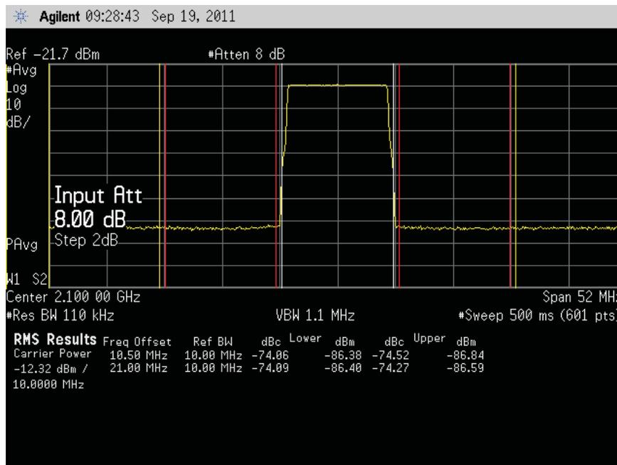
Figure 35. ACPR of 10-MHz LTE Baseband Signal
