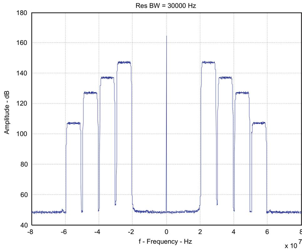
**Figure 29. Four-Carrier QAM256 Pattern Spectral Plot**
