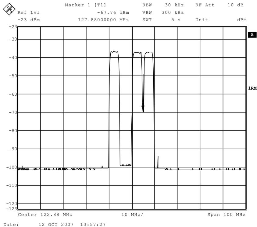
**Figure 27. DAC5687 Output Spectrum for WCDMA TM1 Example**
