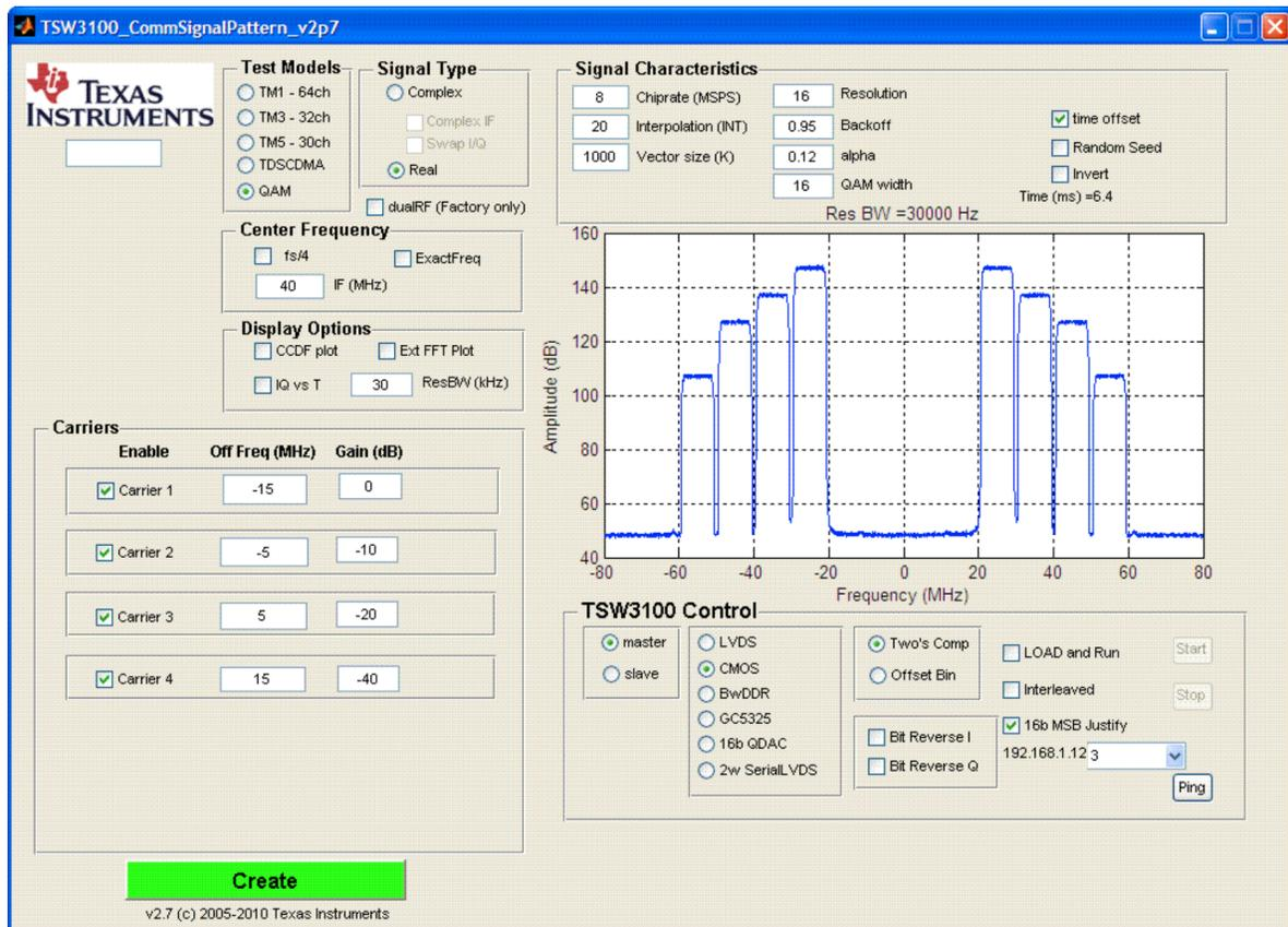
Figure 28. GUI Interface for the Four-Carrier QAM256 Pattern
