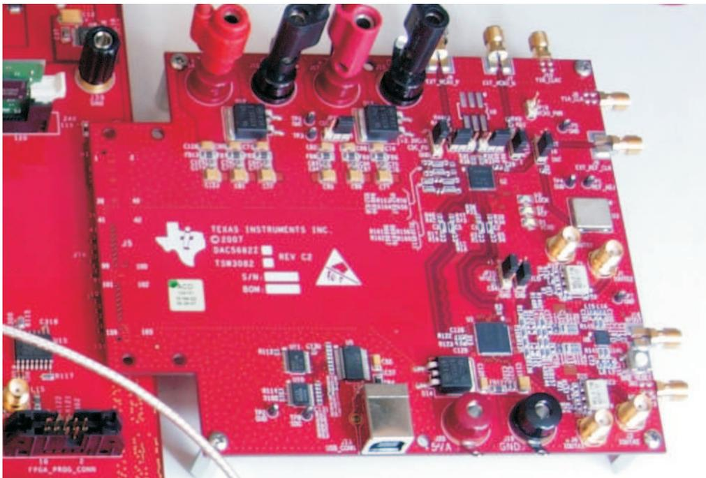
**Figure 13. Connection of the DAC5682Z EVM to the TSW3100**
