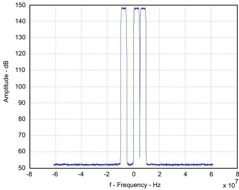
Figure 25. FFT of Three-Carrier WCDMA TM1 Pattern
