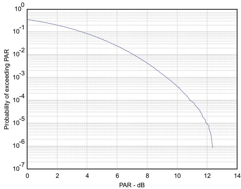
Figure 26. CCDF of Three-Carrier WCDMA TM1 Pattern
