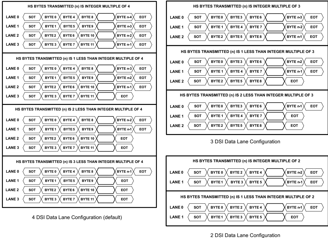
Figure 13. SN65DSI85-Q1 DSI Lane Merging Illustration
