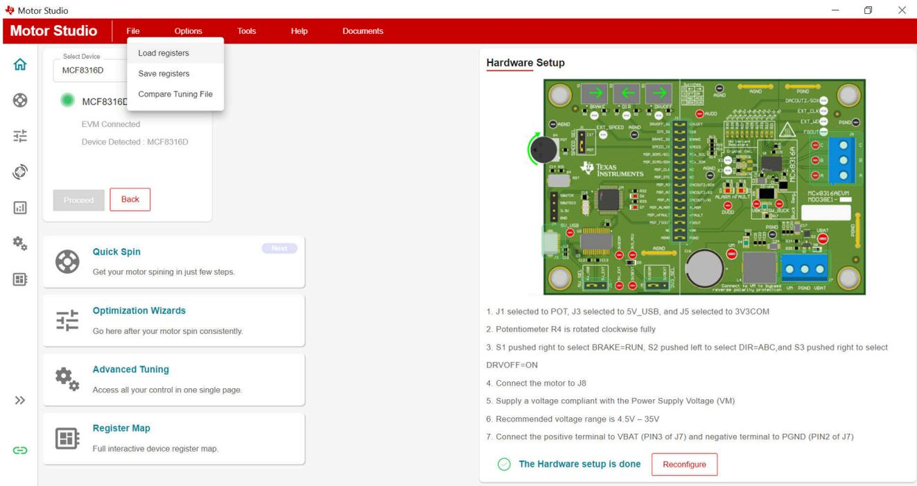
**Figure 3-2. Loading Registers From .json File**
