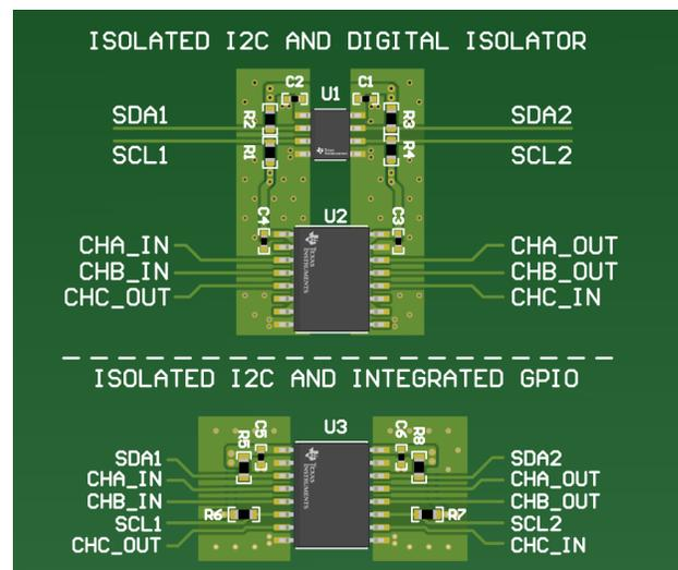
**Figure 1. I2C Footprint of Discrete I2C and Digital Isolator Circuit vs. ISO1644 Isolator Circuit**
