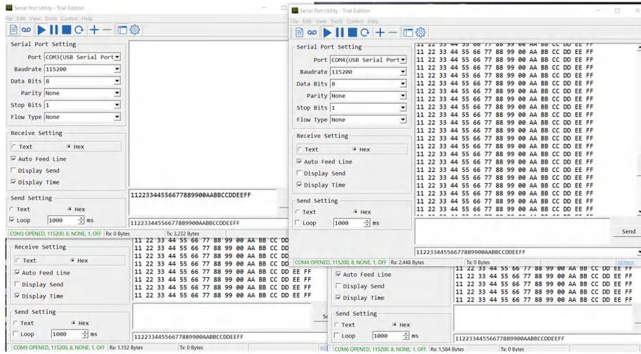
**Figure 2-6. GUI of 4-COM Ports of the 4-Node Terminated Star Network**
