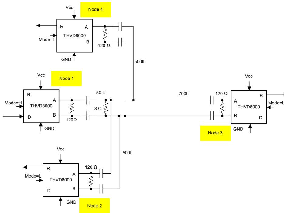
Figure 2-7. 4-Node Loaded and Terminated Star Network
