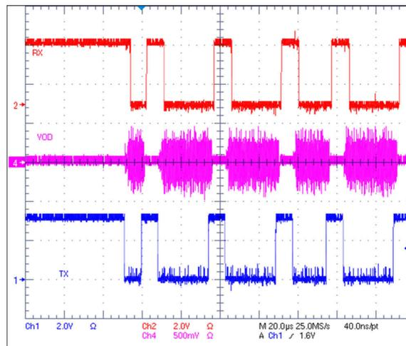
**Figure 2-5. Waveforms of 4-Node Terminated Star Network**
