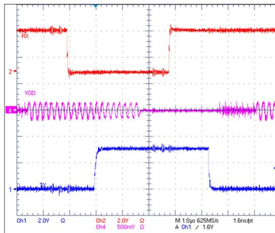
Figure 2-8. Waveforms of the 4-Node Loaded and Terminated Star Network
