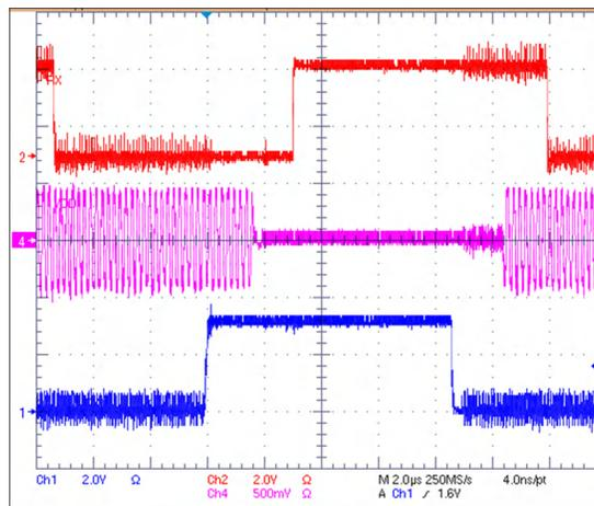
Figure 2-10. Waveforms of the 4-Node Loaded and Terminated Star Network with Line Driver
