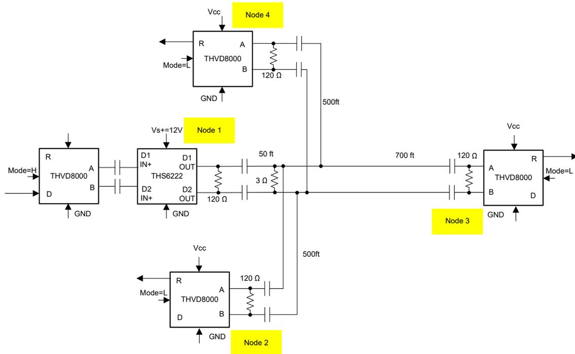
Figure 2-9. 4-Node Loaded and Terminated Star Network with Line Driver
