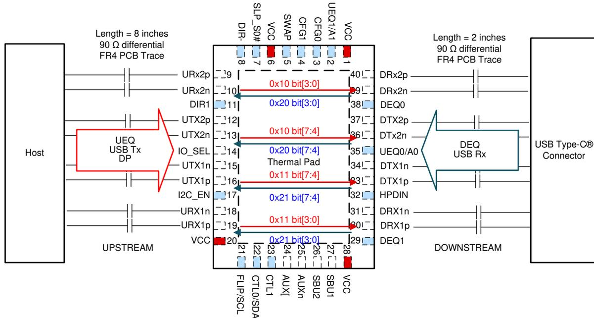
**Figure 2-2. Reference Block Diagram for TUSB1044 Equalization Control**
