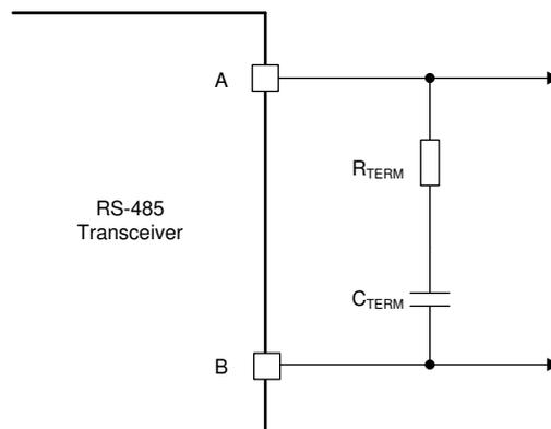
**Figure 6-3. AC Termination Network**
