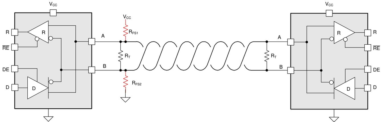
**Figure 5-2. Fail-Safe Resistor Placement**
