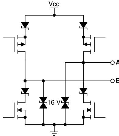
Figure 2-1. Differential Output Driver Structure
