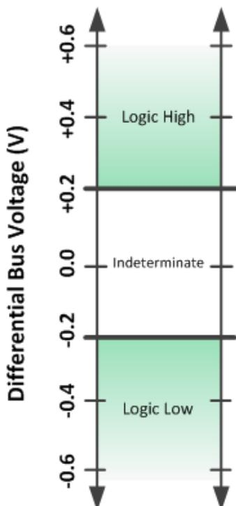
**Figure 5-1. RS-485 Receiver Input Thresholds**
