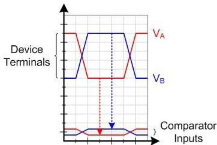
Figure 4-2. Receiver Input-Voltage Attenuation
