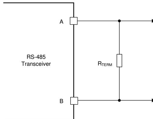
**Figure 6-2. Standard Termination Network**
