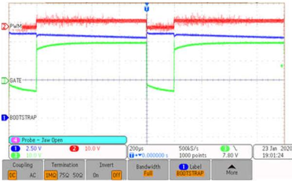
Figure 5-9. Bootstrap Voltage at 1 kHz
