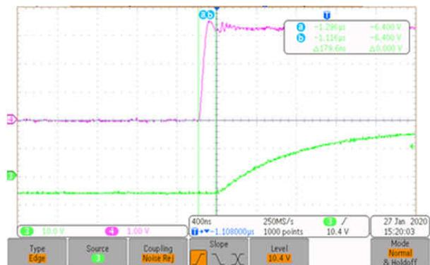
Figure 5-6. Board 2 Propagation Delay Start of Input to Start of Output
