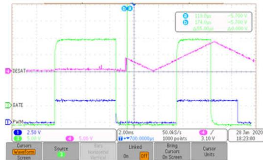
Figure 5-14. DESAT Turn off With R16 and C20
