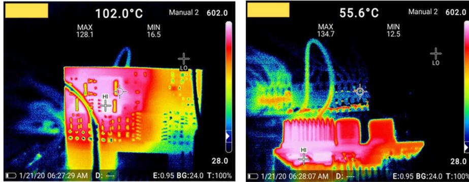
Figure 5-7. Board 1 Thermal Profile
