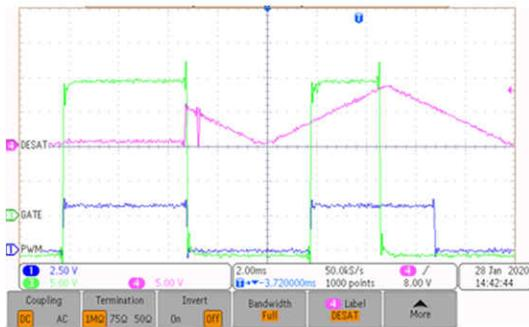
Figure 5-13. DESAT Turn off Without R16 and C20
