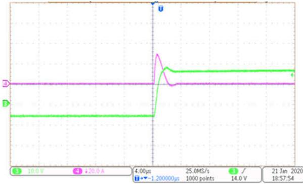
Figure 5-1. Drive-Current Waveform (Board 1)
