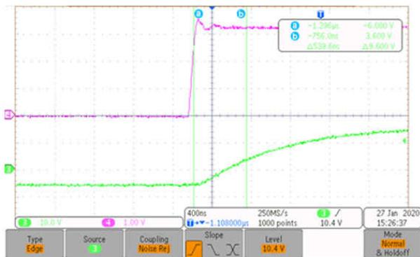
$V_{IH}$  is the logic threshold of the input PWM and the  $V_{TH}$  is the FET typical threshold.
