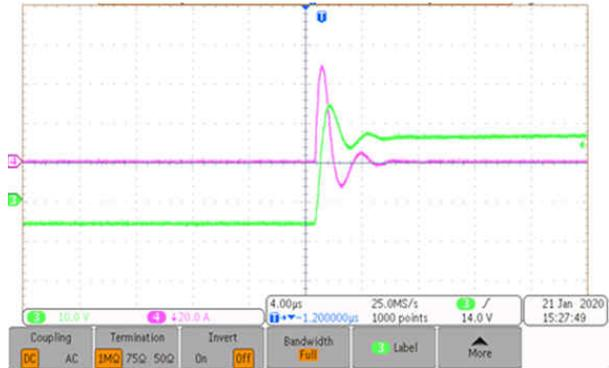
Figure 5-2. Drive-Current Waveform (Board 2)
