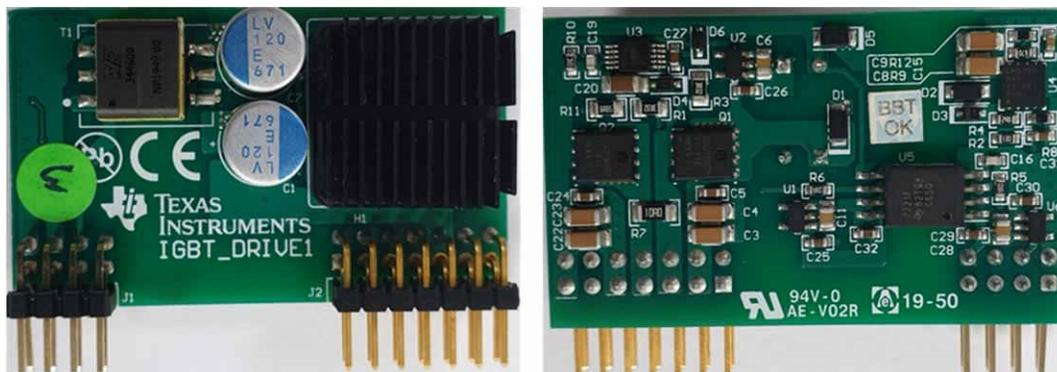
**Figure 4-2. High-Current Gate Driver Board Using LM5106 and MOSFETs (Top and Bottom View)**
