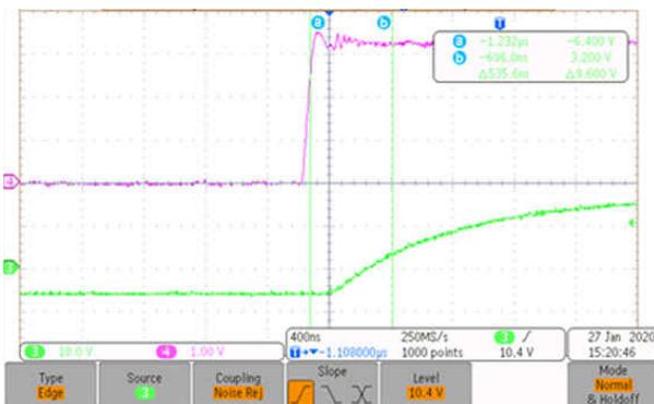
Figure 5-5. Board 2 Propagation Delay  $V_{IH}$  to  $V_{TH}$
