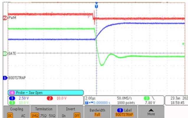
Figure 5-11. Bootstrap Voltage Charging Time
