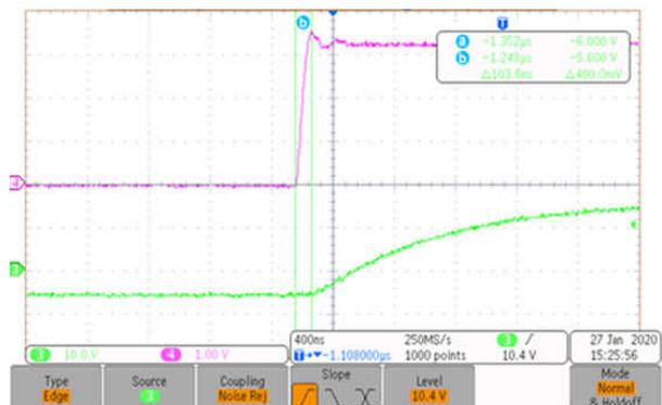
Figure 5-4. Board 1 Propagation Delay Start of Input to Start of Output
