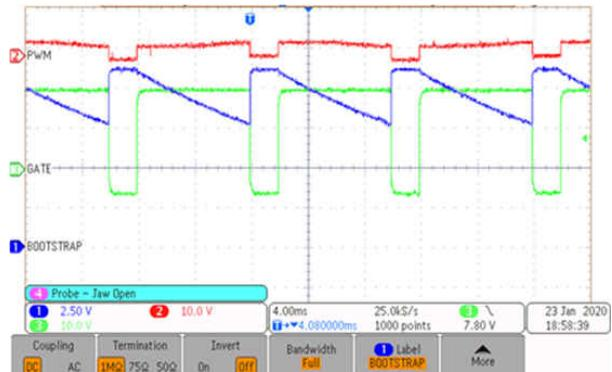
Figure 5-10. Bootstrap Voltage at 100 Hz
