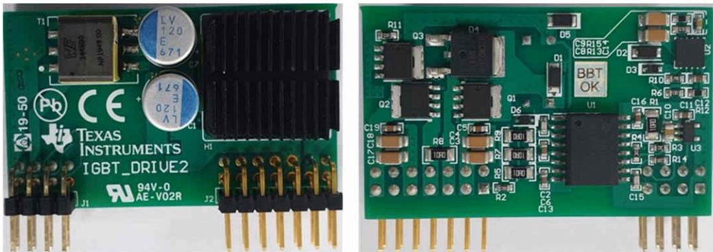
**Figure 4-1. High-Current Gate-Driver Board Using ISO5852S and BJTs (Top and Bottom View)**
