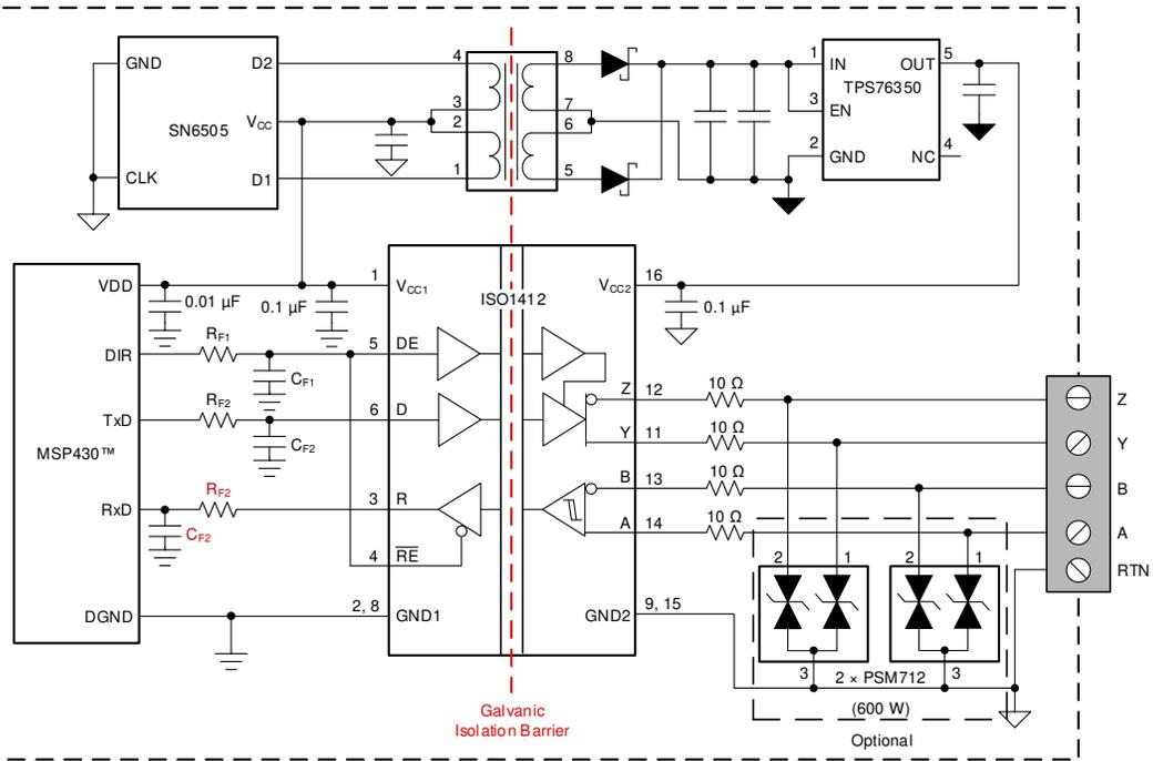
**Figure 1-2. Full-duplex Isolated RS-485 Node**
