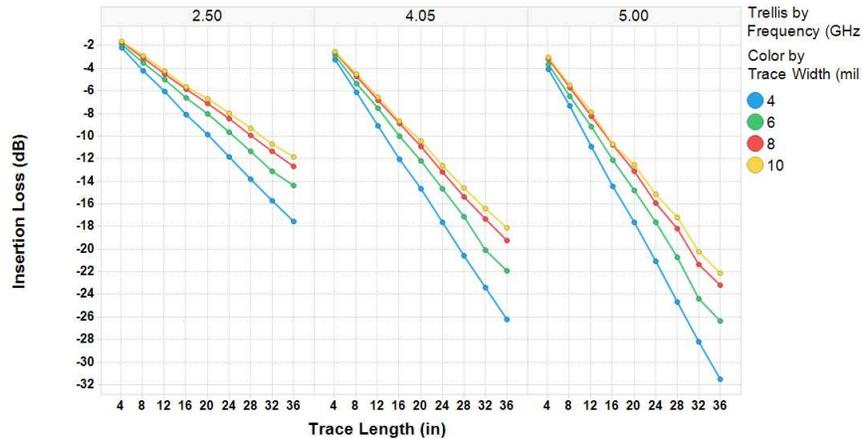
Figure 7. PCB Trace Insertion Loss vs. Signal Frequency
