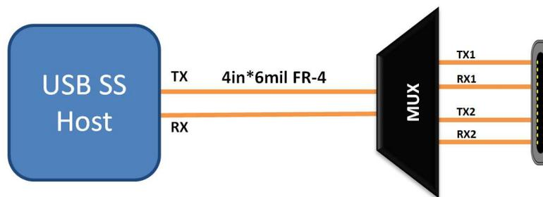
Figure 10. Illustration of a Small System Such as a Smartphone
