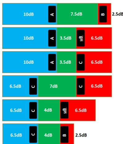
Figure 5. USB 3.1 Gen 1 5Gbit/s Insertion Loss Budget
