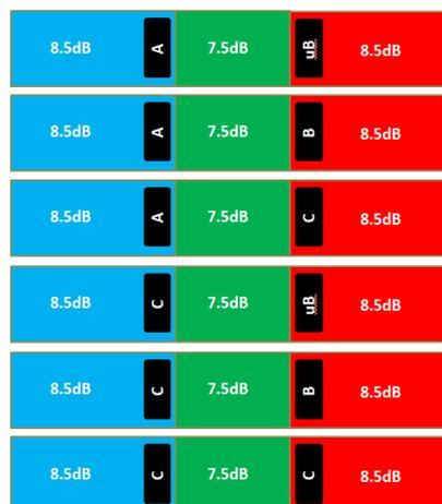
Figure 6. USB 3.1 Gen 2 10Gbit/s Insertion Loss Budgets
