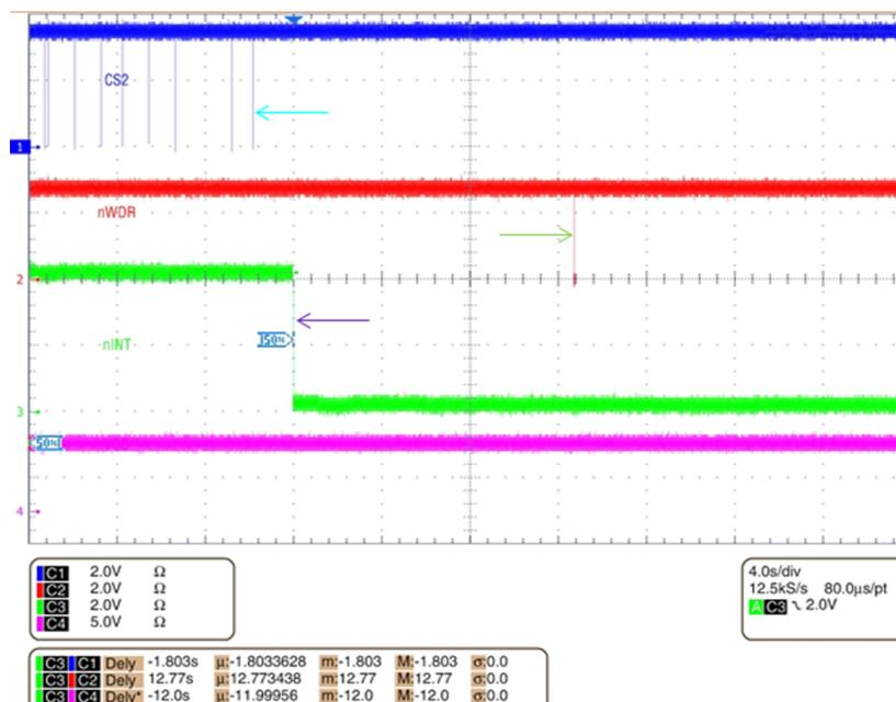
Figure 4. TLIN14415-Q1 Window Watchdog Service and Failure
