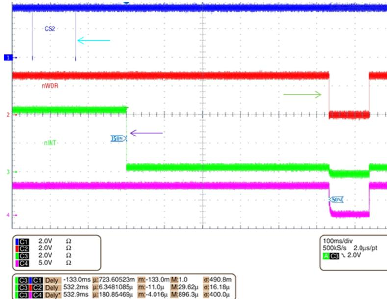
Figure 5. TLIN14415-Q1 Timeout Watchdog Service and Failure
