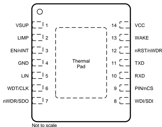
**Figure 1. TLINx441x Pinout**
