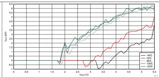
Figure 18. 3.3 V LDO Sleep Mode Ramp Down
