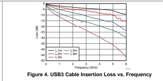
Figure 4. USB3 Cable Insertion Loss vs. Frequency
