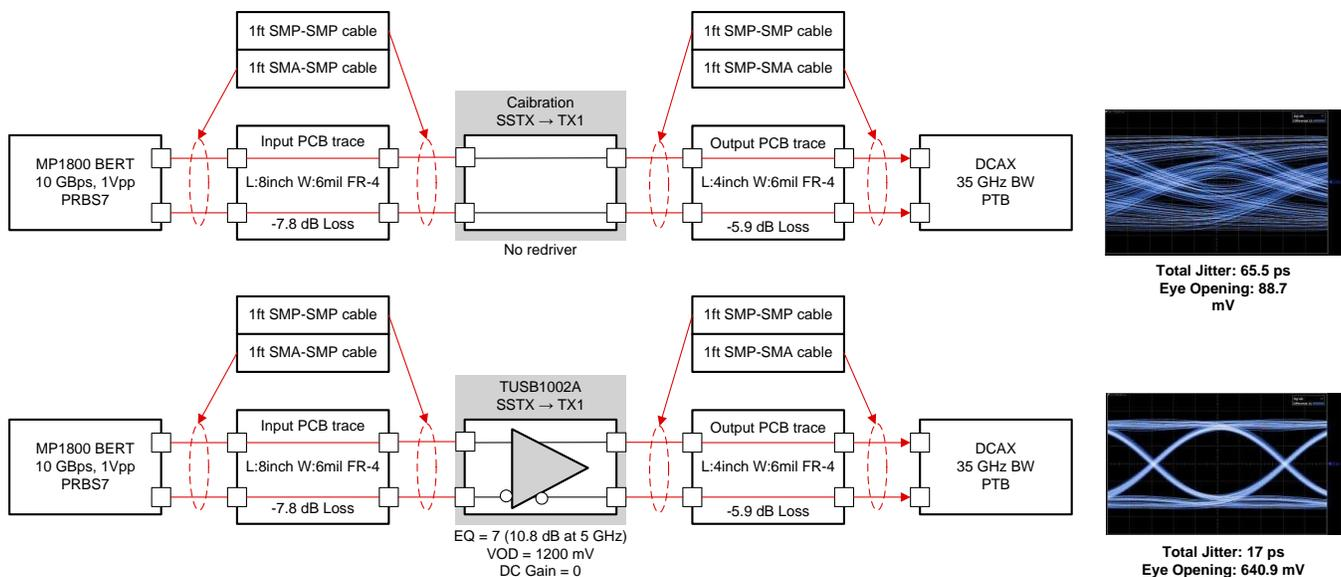
Figure 1. Comparison Between With and Without Redriver
