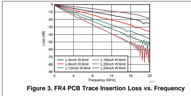
Figure 3. FR4 PCB Trace Insertion Loss vs. Frequency
