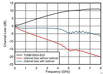
Figure 14. Channel Loss Frequency Response Curve
