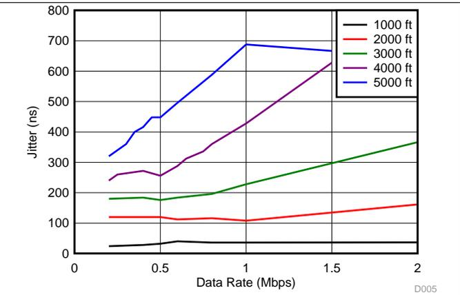
Figure 6. A-B Bus Jitter vs Data Rate
