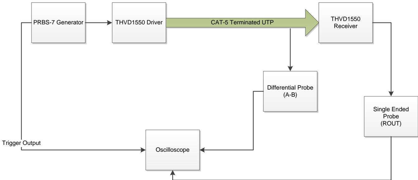
Figure 4. Lab Setup
