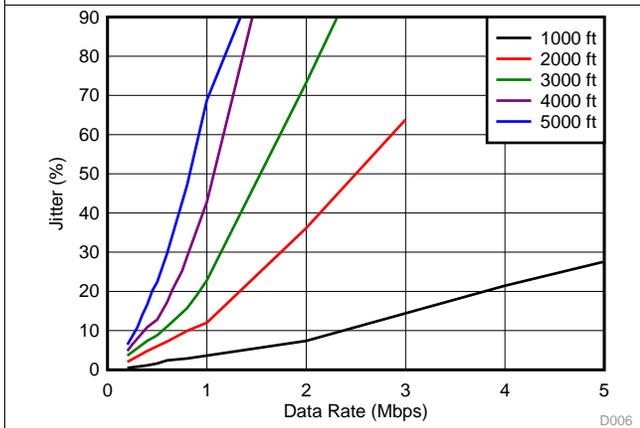
Figure 7. A-B Bus Jitter % vs Data Rate
