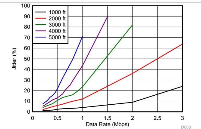
Figure 10. Receiver Jitter % vs Data Rate
