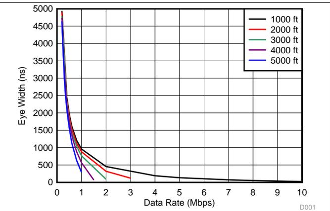
Figure 8. Receiver Eye Width vs Data Rate
