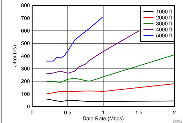
Figure 9. Receiver Jitter vs Data Rate
