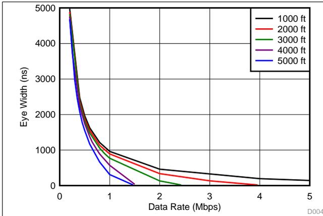
Figure 5. A-B Bus Eye Width vs Data Rate
