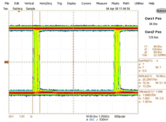
**Figure 3. Actual Receiver Output after 1000 ft at 3 Mbps**
