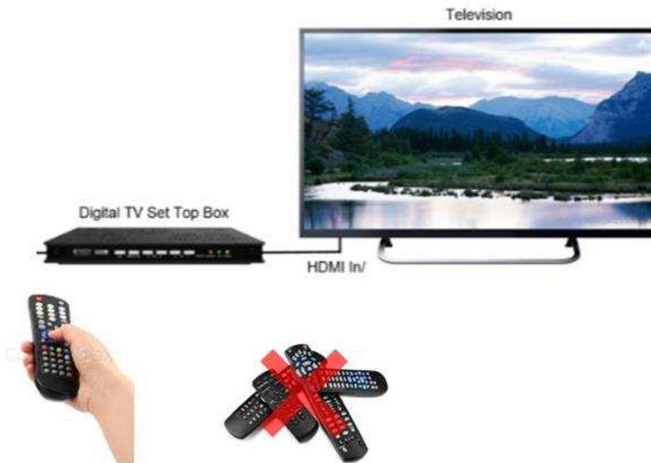
**Figure 8. Single Remote Controller for Both HDMI Sink and Source**
