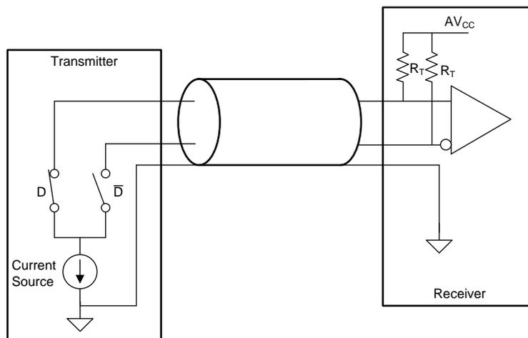
Figure 2. Conceptual Schematic for one TMDS Differential Pair
