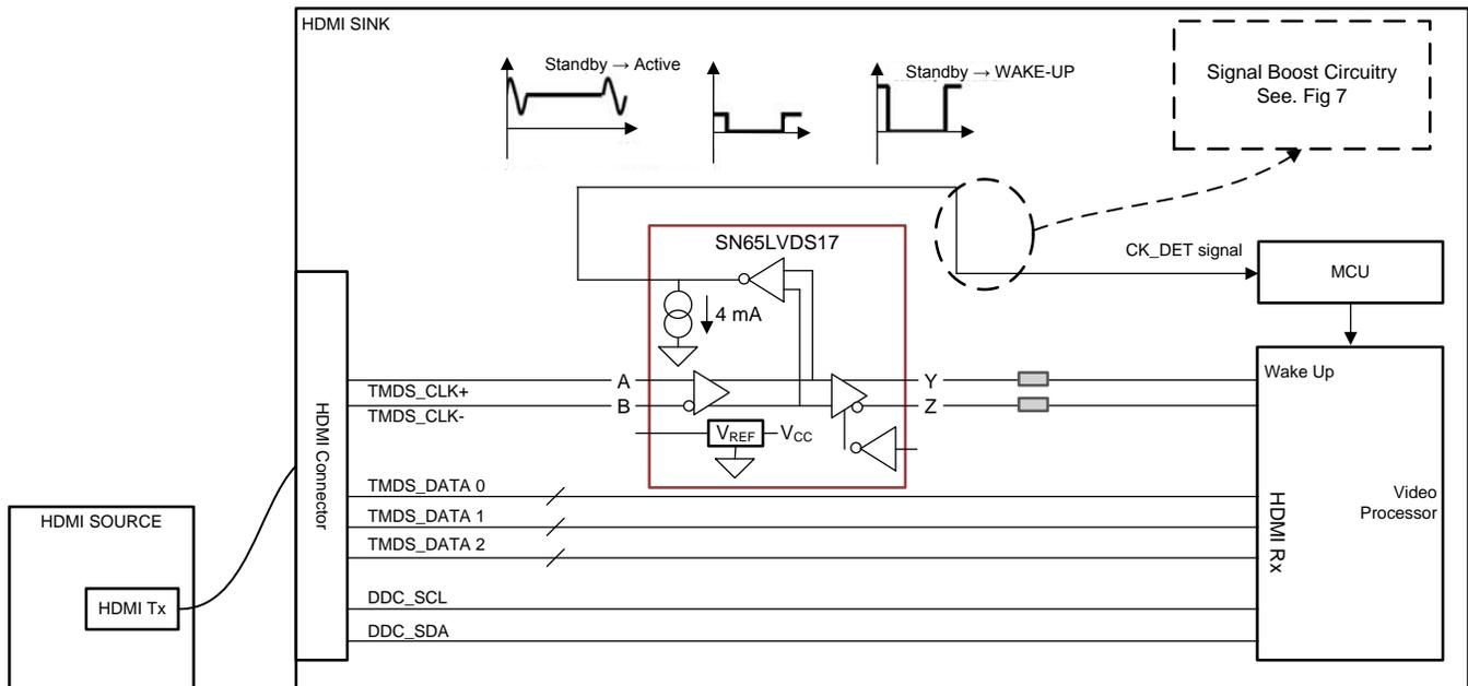
Figure 4. Implementation Example Block Diagram 2 - Single-Chip Implementation
