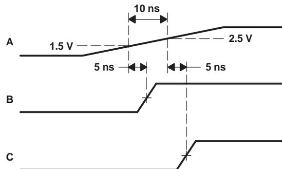
**Figure 6. Incorrect Operation of a Shift Register**
