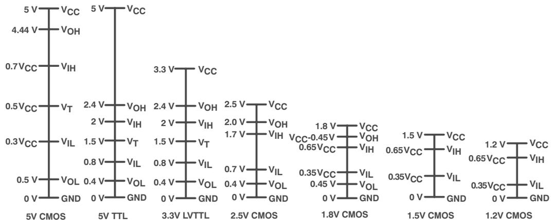
Figure 4. Common Switching Input and Output Levels
