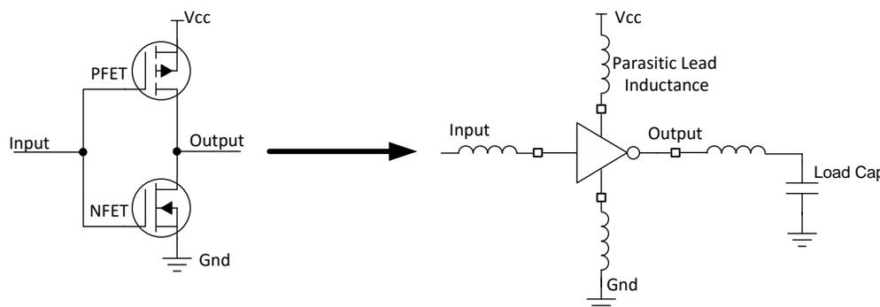
Figure 2. Parasitic lead Inductances associated with the package
