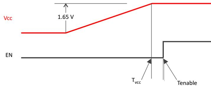
Figure 2. Cold Start Vcc Ramp Up to EN
