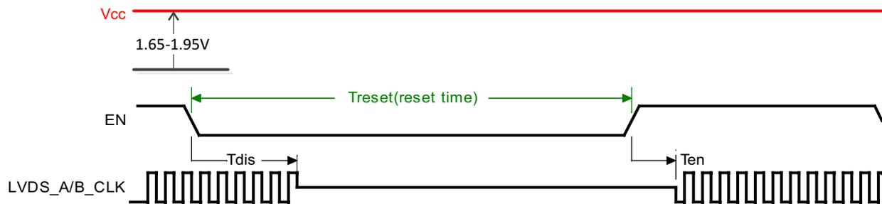
Figure 3. RESET or SHUTDOWN Timing When Vcc = HIGH
