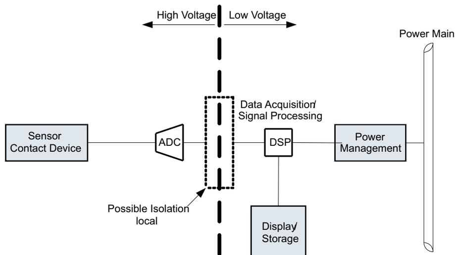
**Figure 2. Isolation Between High-Voltage and Low-Voltage Circuits**
