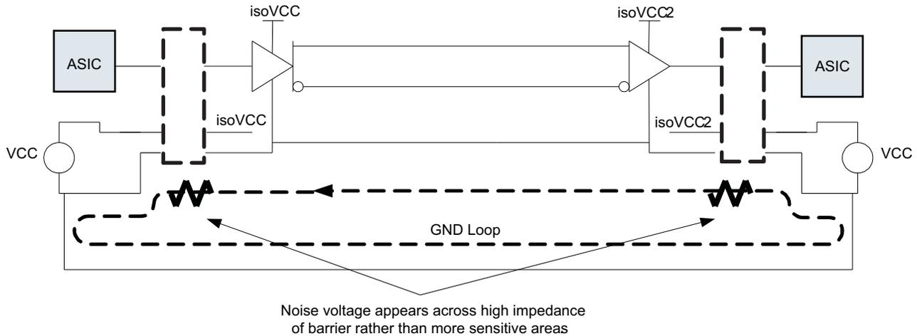
**Figure 4. Ground Loops Between Nodes Broken With Isolation**
