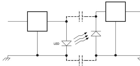
**Figure 11. Barrier Capacitance**
