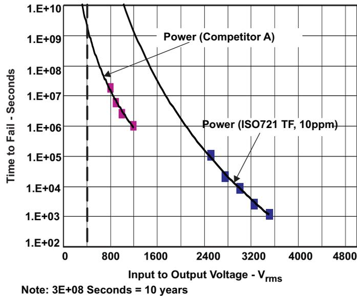
**Figure 4. High-Voltage Lifetime Based on Best Curve Fit**
