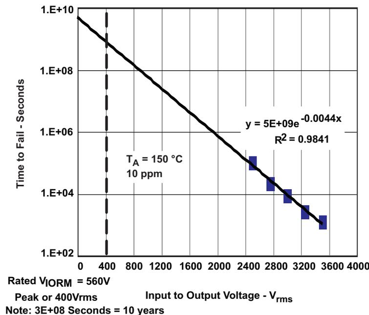
Figure 3. High-Voltage Lifetime Using TDDB E Model
