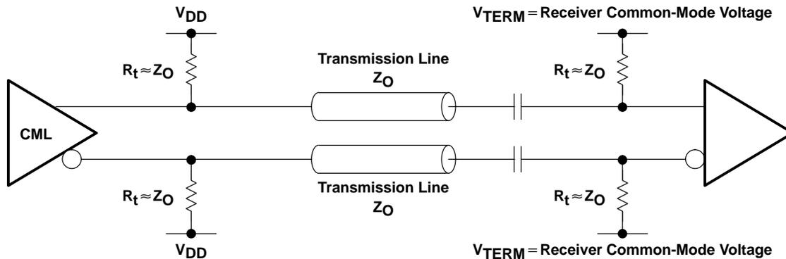
**Figure 13. CML Driver for AC-Coupling**
