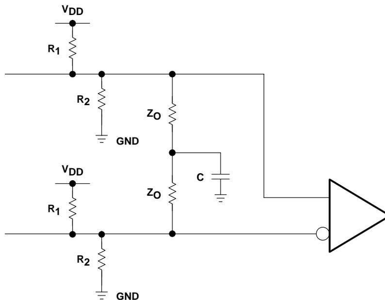
**Figure 21. Differential Termination With Biasing and Decoupling Capacitor**
