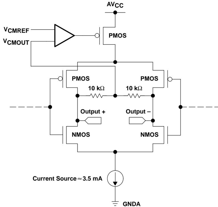
Figure 8. Typical Structure for an LVDS Output Stage
