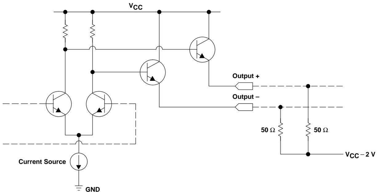
Figure 2. Typical Structure for an LVPECL Output Stage
