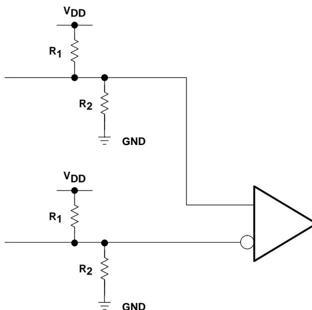
**Figure 22. Differential Termination With Reduced Resistor Count**
