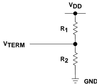
Figure 18. Simple Resistor Network for Biasing Voltages
