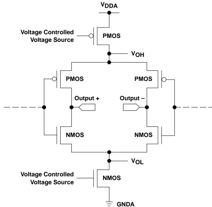
Figure 6. Typical Structure for a VML Output Stage
