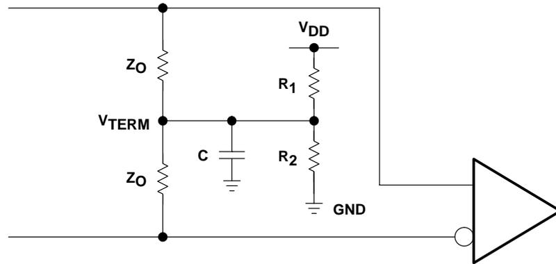
Figure 24. Differential Termination With One Biasing Network
