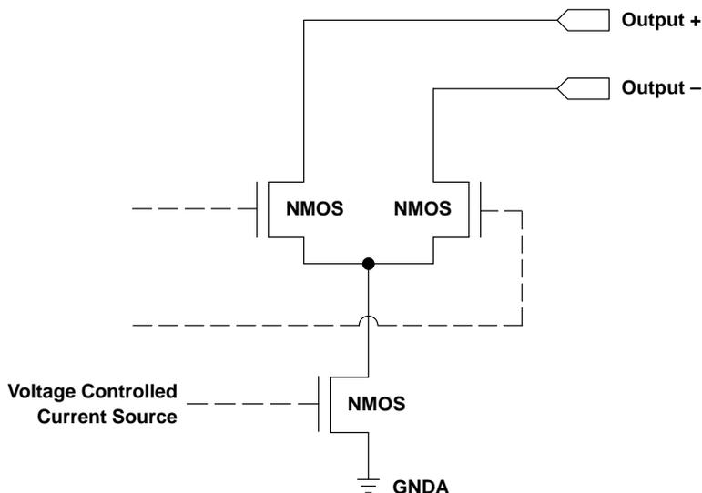
Figure 4. Typical Structure for a CML Output Stage
