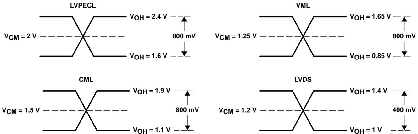
**Figure 1. Graphic Voltage Swings by Logic Level**
